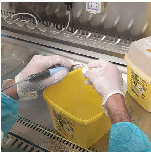
FIGURE 2 Operator while using piezoelectric ultrasonic scalpel (PUS) to remove biofilm from a disk under the laminar flow hood.
