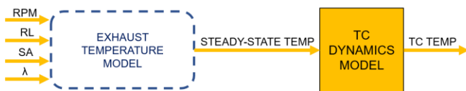
Figure 19. The exhaust manifold temperature model was coupled with the TC dynamic model in order to reproduce the TC signal also under transient conditions.
