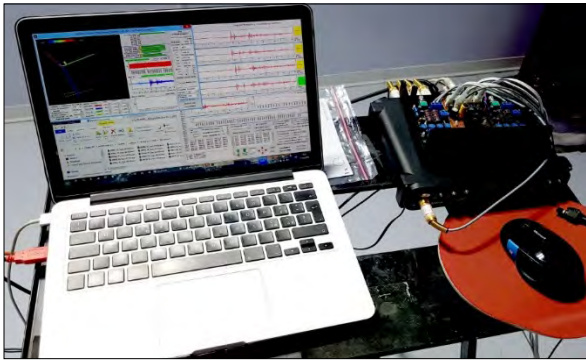
Figure 3. Measurement system. PC and amplifiers.
