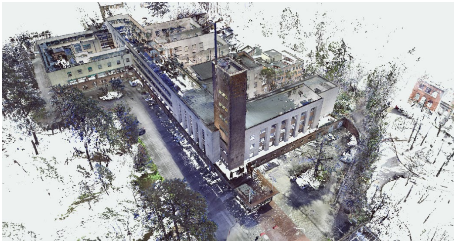
Fig. 14. Screenshot with the entire point cloud model of the Faculty of Engineering of Bologna in FARO SCENE software. (authors' digital elaboration)
