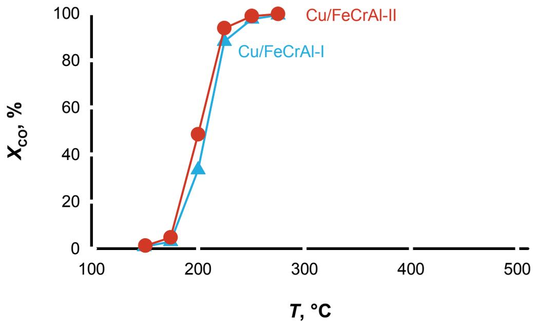
Figure 24: CO conversion vs. temperature: for bulk metal fibers (above) and for Cu-coated FeCrAl fibers (below). Adapted with permission from reference.<sup>188</sup> Copyright 2018 Elsevier.
