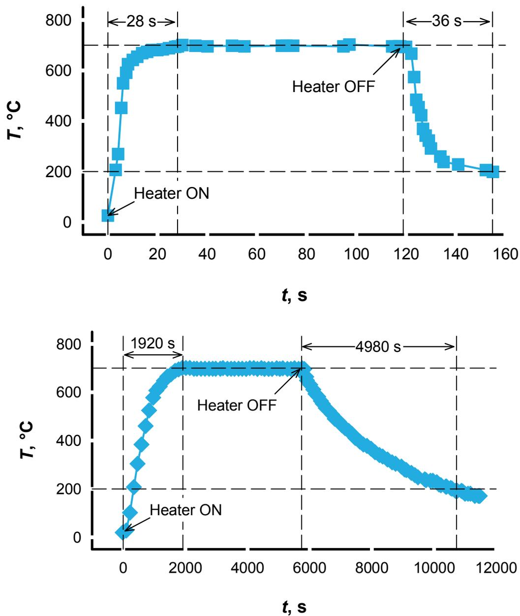
Figure 38: Catalyst temperature profile vs time for electrified support (top) and outside heated (bottom).<sup>245</sup> Copyright 2011 Elsevier.
