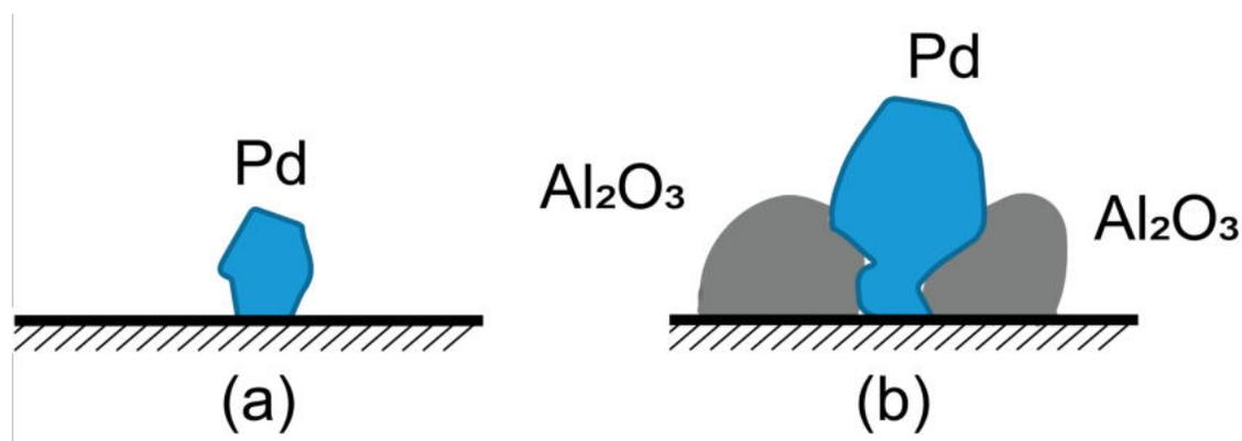
Figure 33: Electroplated palladium particles on virgin (a) and oxidized (b) FeCrAl substrate. Adapted with permission from reference.<sup>233</sup> Copyright 2017 American Chemical Society.
