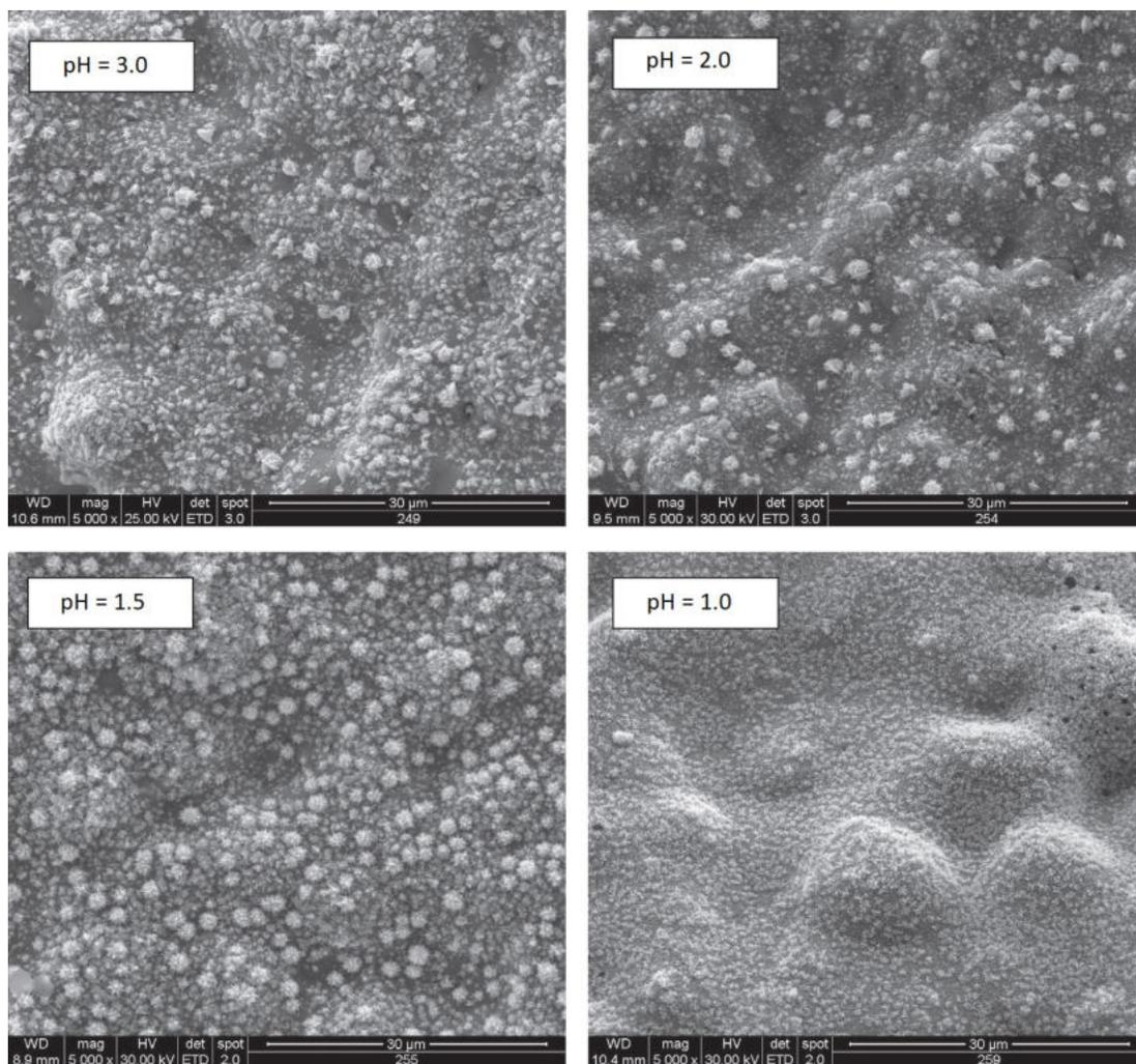
Figure 19: SEM micrographs of FeCrAl foams obtained by spontaneous deposition of Pd as a function pH. Adapted with permission from reference.<sup>153</sup> Copyright 2013 Elsevier.
