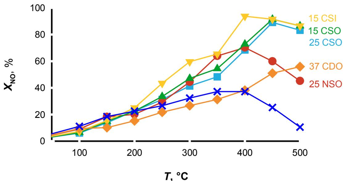
Figure 25: NO conversion vs temperature of samples (Table 2). Adapted with permission from reference.<sup>146</sup>
