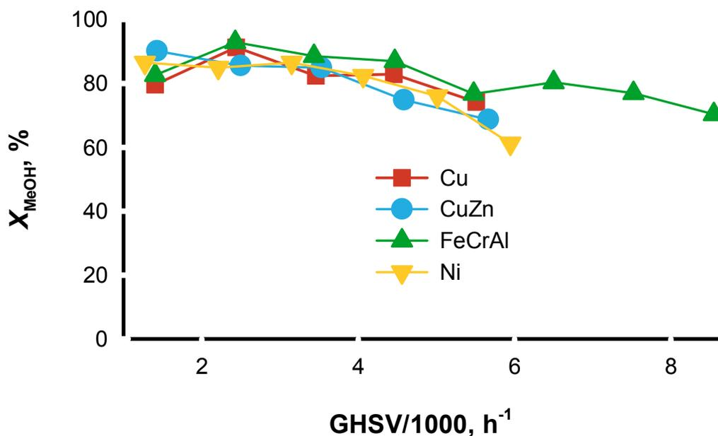
Figure 43: Methanol conversion vs of GHSV on different metal foam.<sup>289</sup> Copyright 2007 Elsevier.
