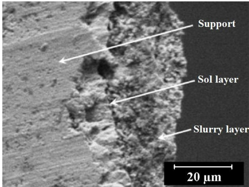
Figure 11: Scanning electron microscope (SEM) image of sample section after 10 h pre-oxidation at 900 °C, sol layer 2%  $\text{g g}^{-1}$  and slurry 25.3%  $\text{g g}^{-1}$  deposition. Adapted with permission from reference.<sup>120</sup> Copyright 2017 Elsevier.
