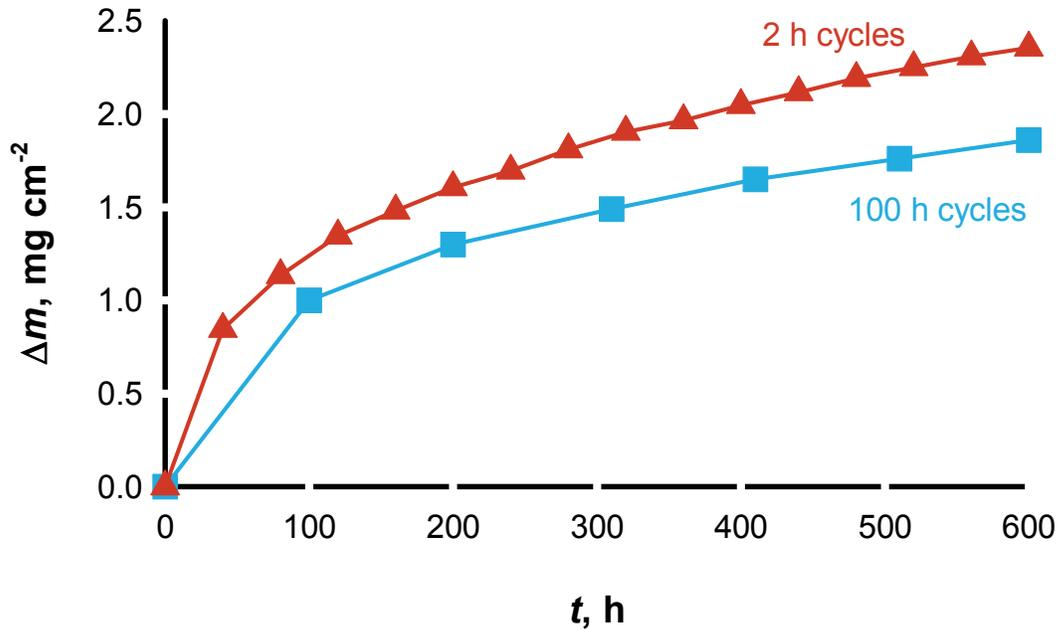
Figure 10: Mass increase depending on the air oxidation cycle duration at 1200 °C. Adapted with permission from reference.<sup>100</sup> Copyright 2004 Springer Nature.
