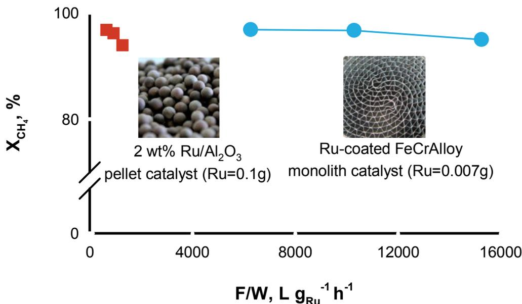
Figure 39: Conversion vs space velocity (flow over weight  $F/W$ ) over commercial 2% Ru/Al<sub>2</sub>O<sub>3</sub> pellet and Ru-coated FeCrAl monolith in SMR at 700 °C,  $S/C = 3.0$ ,  $F/W = 430 \text{ L g}^{-1} \text{ h}^{-1}$  to  $15\,100 \text{ L g}^{-1} \text{ h}^{-1}$ .<sup>250</sup> Copyright 2017 Elsevier.
