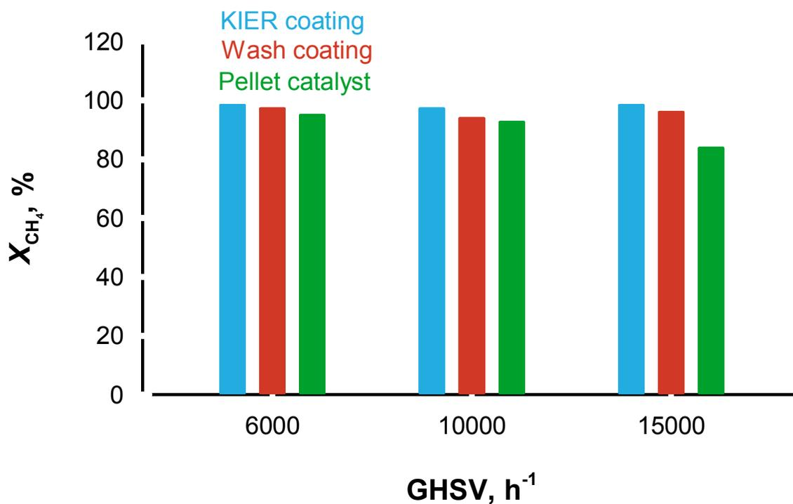
Figure 37:  $\text{CH}_4$  conversion vs GHSV for  $\text{Ni}/\text{MgAl}_2\text{O}_4$  catalyst. Adapted with permission from reference.<sup>241</sup> Copyright 2016 Elsevier.
