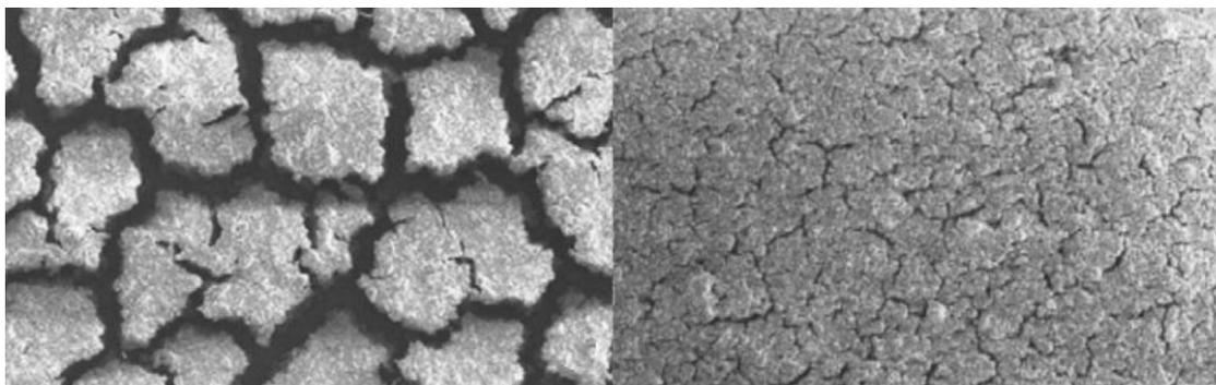
Figure 14: FeCrAl surface micrographs after 2 h at 1200 °C. With (right) and without (left) 2% g g<sup>-1</sup> La. Adapted with permission from reference.<sup>126</sup> Copyright 2015 Elsevier.
