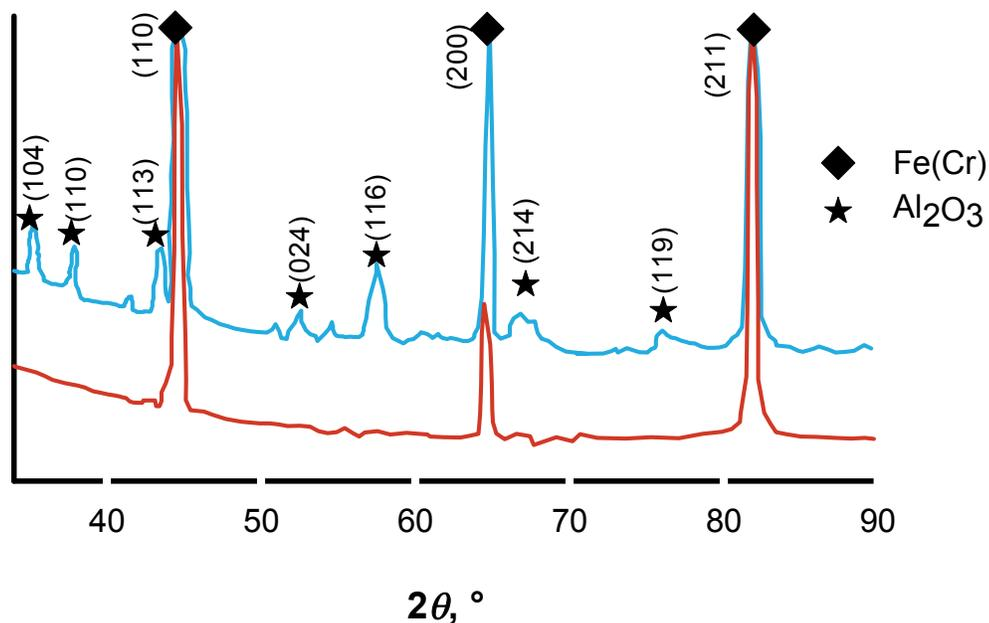
Figure 8: X-ray diffraction (XRD) analysis of FeCrAl before (red) and after (blue) preoxidation. Adapted with permission from reference.<sup>97</sup> Copyright 2012 Elsevier.
