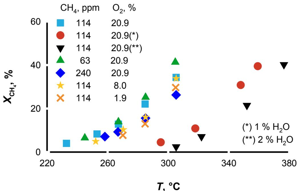
Figure 28: CH<sub>4</sub> conversion vs temperature as a function of co-reactant (O<sub>2</sub> and H<sub>2</sub>O) concentration. Adapted with permission from reference.<sup>211</sup> Copyright 2015 Elsevier.
