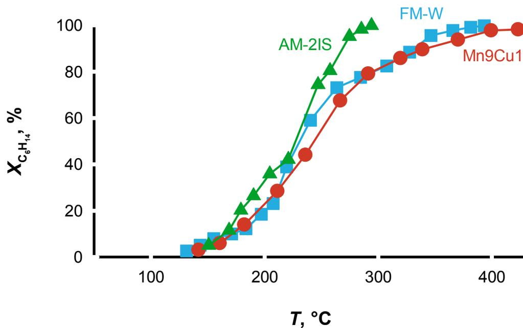
Figure 35: Conversion of toluene (top) and n-hexane vs. reaction temperature on FeCrAl washcoated monolith, impregnated AM-2IS and powder  $Mn_9Cu_1$  catalyst. Adapted with permission from reference.<sup>231</sup> Copyright 2011 Springer Nature.
