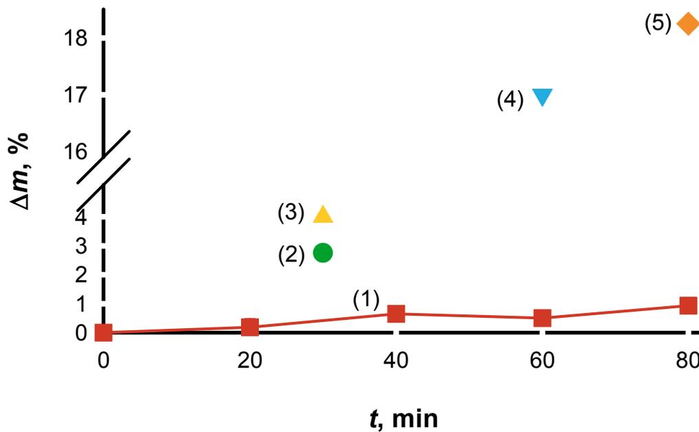
Figure 13: Weight loss comparison during mechanical stress test at 40 kHz in ultrasonic bath. (1),<sup>97</sup> (2),<sup>114</sup> (3),<sup>110</sup> (4)<sup>124</sup> and (5).<sup>120</sup> Adapted with permission from reference.<sup>97</sup> Copyright 2012 Elsevier.
