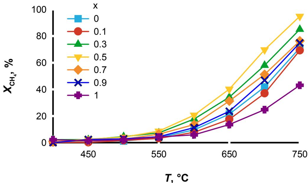
Figure 29: Methane conversion vs temperature over  $\text{LaFe}_{1-x}\text{Mg}_x\text{O}_3/\text{Al}_2\text{O}_3/\text{FeCrAl}$  catalysts. GHSV =  $36\,000\text{ mL g}^{-1}\text{ h}^{-1}$ . Adapted with permission from reference.<sup>220</sup> Copyright 2006 Elsevier.
