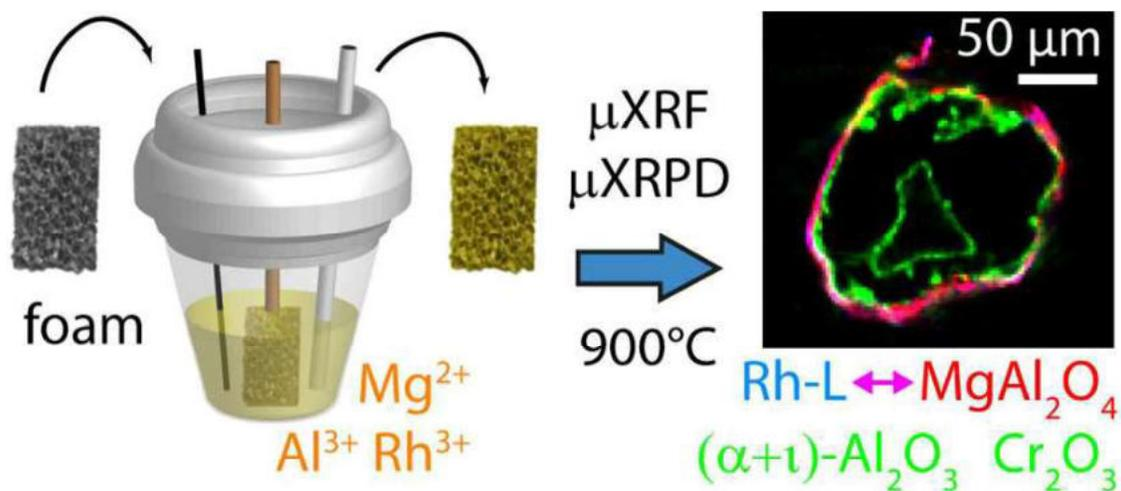
Figure 41: Production method and micrograph of electro-synthesized Rh foam. Adapted with permission from reference.<sup>167</sup> Copyright 2014 American Chemical Society.
