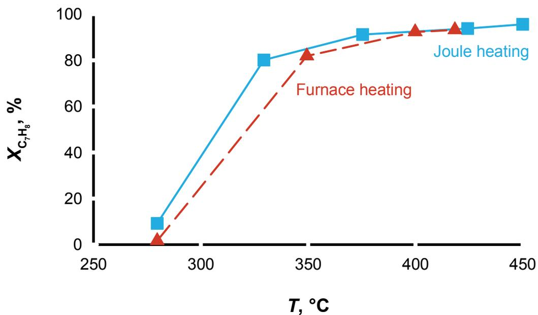
Figure 34: CO and C<sub>7</sub>H<sub>8</sub> conversion over Mn supported FeCrAl wire as a function of heating methods. Adapted with permission from reference.<sup>111</sup> Copyright 2017 Elsevier.
