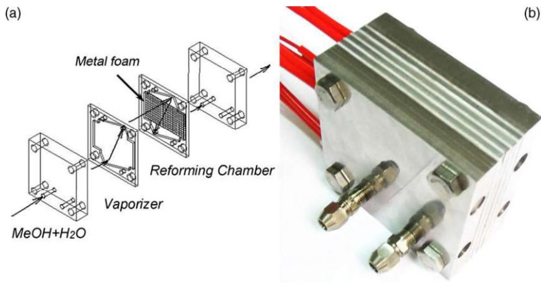
Figure 44: Reactor mechanical drawing: (a) integrated operative reactor (b).<sup>289</sup> Copyright 2007 Elsevier.
