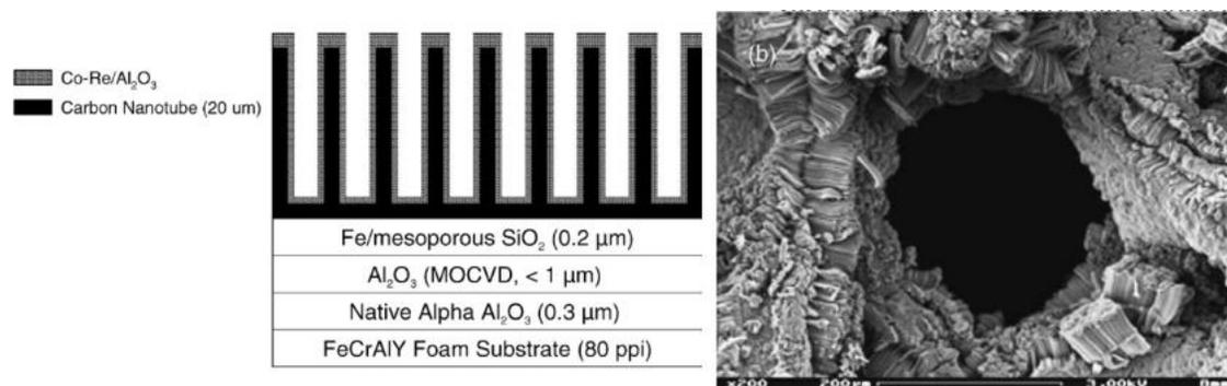
Figure 45: Schematic of engineered catalyst based on multilayer carbon nanotube arrays for Fischer-Tropsch synthesis in a microchannel reactor (left). Micrograph of the prepared foam (right).<sup>314</sup> Copyright 2005 Elsevier.
