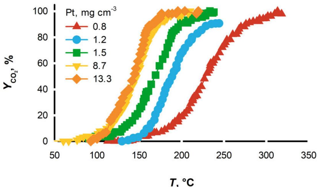
Figure 31: Methanol yield to CO<sub>2</sub> vs reaction temperature over Pt/FeCrAl foam catalysts at increasing Pt loading. Feed conditions: CH<sub>3</sub>OH 0.5% in air, GHSV = 16 500 h<sup>-1</sup>. Adapted with permission from reference.<sup>155</sup> Copyright 2016 Elsevier.
