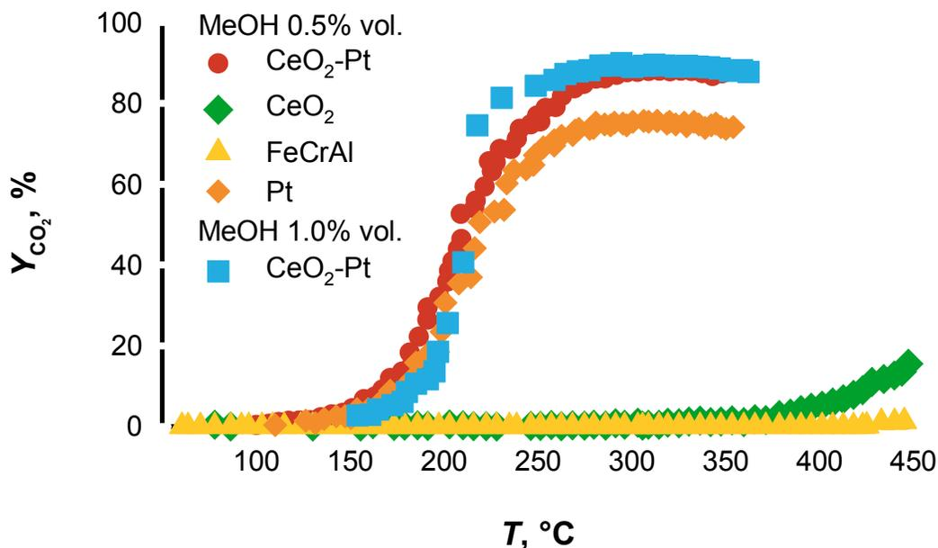
Figure 32: Methanol yield to CO<sub>2</sub> vs reaction temperature over several catalysts. Feed conditions: GHSV = 16 500 h<sup>-1</sup>, CH<sub>3</sub>OH = 0.5% to 1% in air. Adapted with permission from reference.<sup>168</sup> Copyright 2017 Elsevier.
