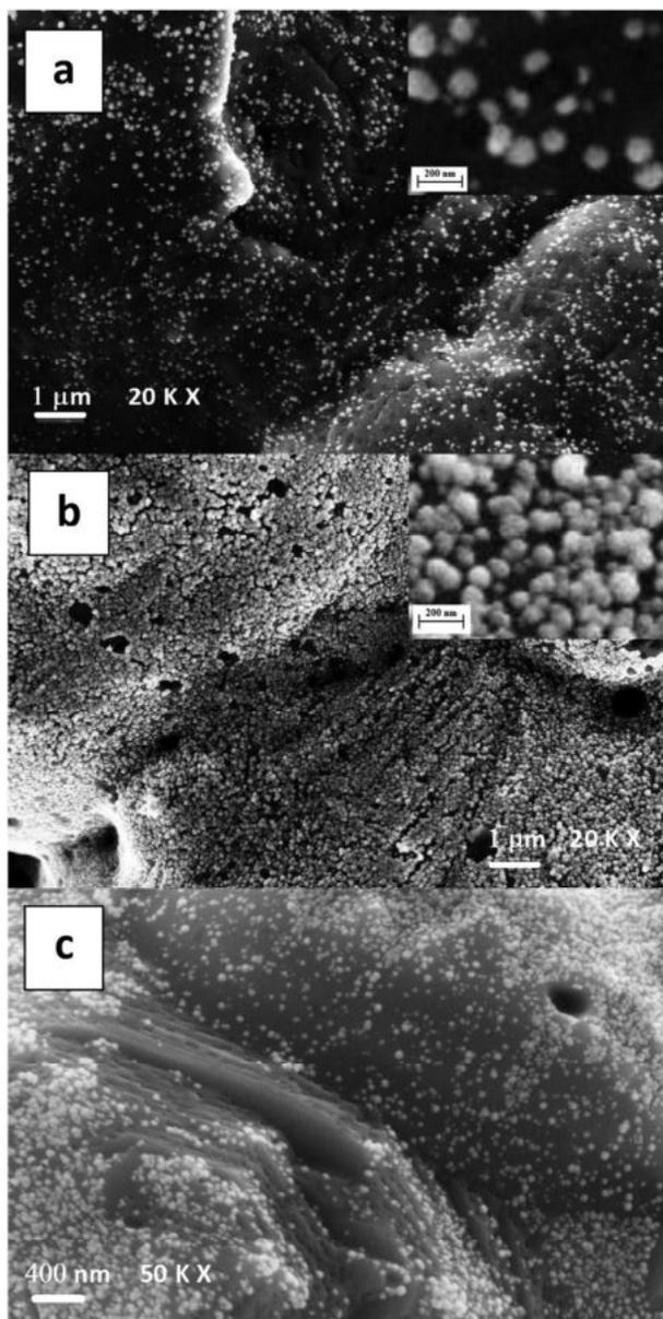
Figure 20: SEM micro-graphs of Rh-FeCrAl samples prepared following electro-deposition (a,b) or spontaneous deposition (c).<sup>154</sup> Copyright 2014 Elsevier.
