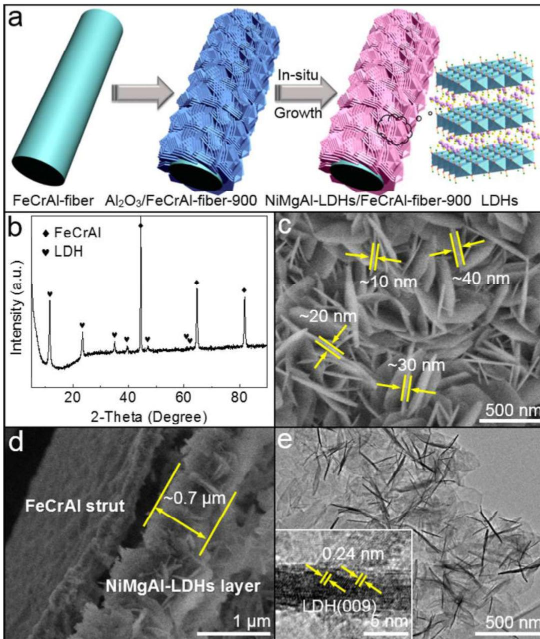
Figure 18: Fabrication strategy (a) of the  $\text{NiO-MgO-Al}_2\text{O}_3/\text{FeCrAl-fiber-900}$  catalyst derived from the  $\text{NiMgAl-LDHs/FeCrAl-fiber-900}$  precursor. XRD pattern (b), SEM (c,d) and TEM micro-graphs (e) of the  $\text{NiMgAl-LDHs/FeCrAl-fiber-900}$  precursor.<sup>88</sup> Copyright 2017 American Chemical Society.
