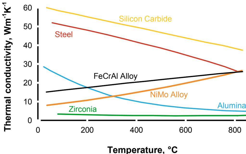
Figure 5: Thermal conductivity vs temperature of some of the most used catalyst supports. Adapted with permission from reference.<sup>72</sup>
