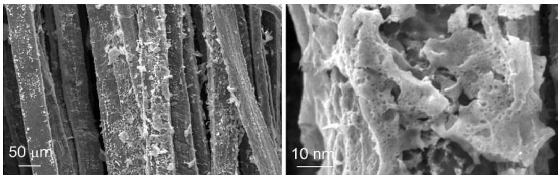
Figure 16: SEM micro-graphs of FeCrAl fibers supporting Pd(LaMnO<sub>3</sub> · 2ZrO<sub>2</sub>) prepared by in situ SCS.<sup>140</sup>
