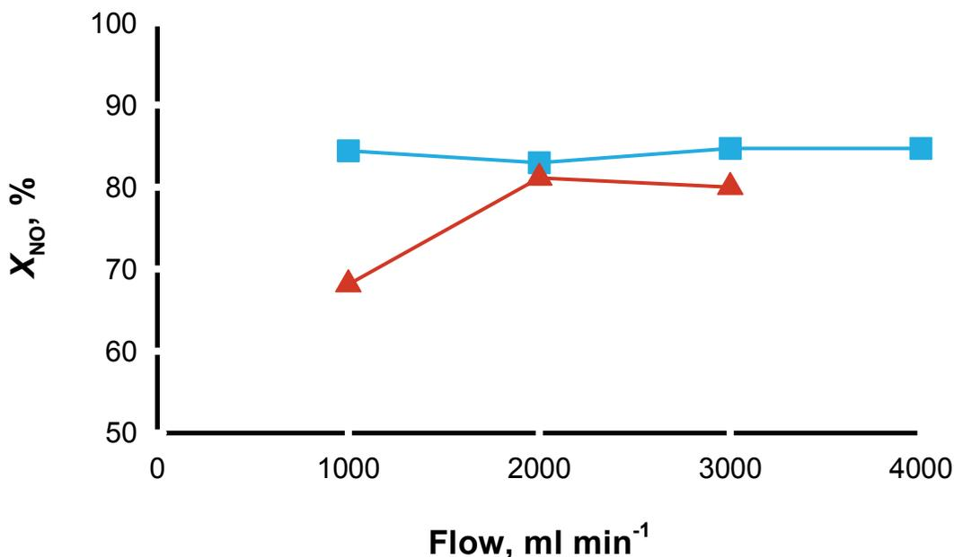
Figure 23: Conversion of NO as function of the residence time for FeCrAl hollow sphere structured bed (blue) and ceramic monolith (red). Adapted with permission from reference.<sup>93</sup> Copyright 2009 Elsevier.
