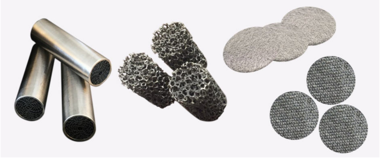
Figure 4: Most common examples of FeCrAl structures. Monoliths, foams and fibers (random sintered or knitted). Adapted with permission from reference. 53
