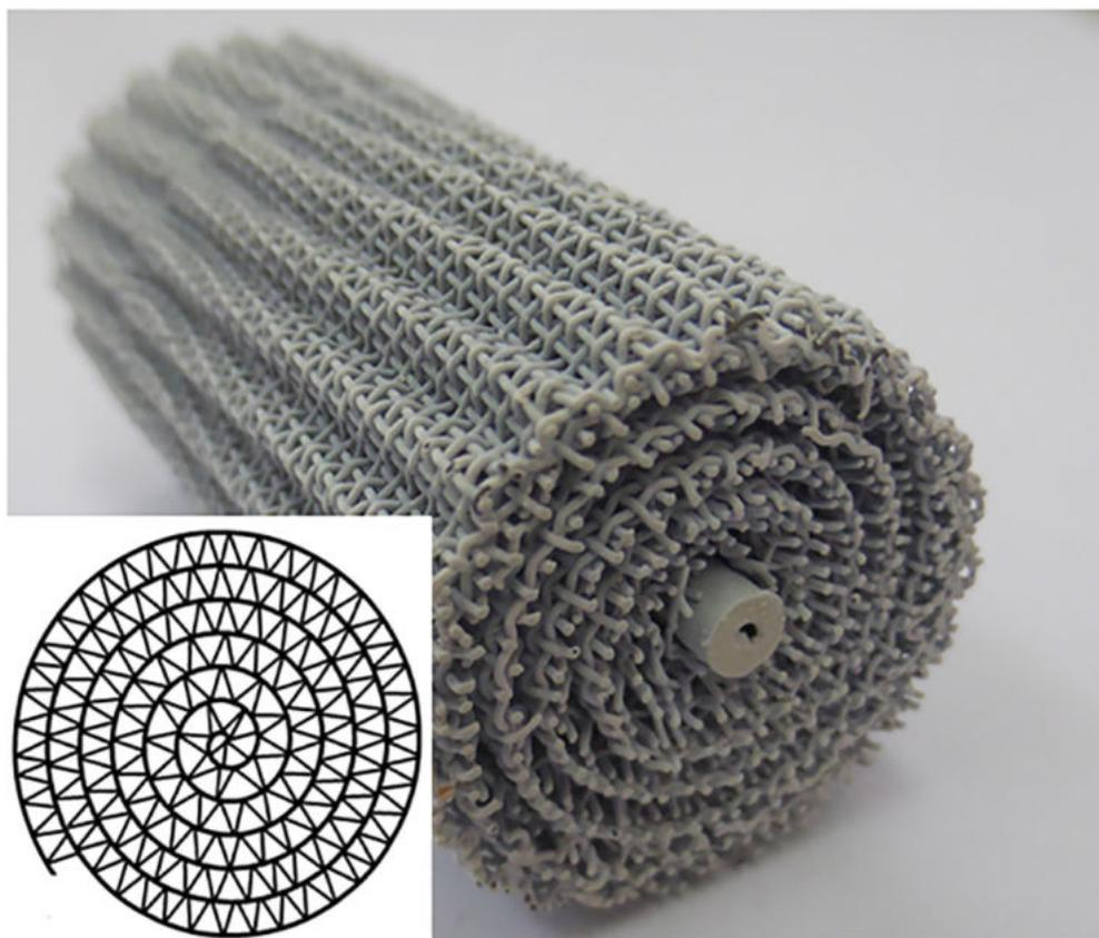
Figure 42: Structured catalyst overview and cross section.<sup>268</sup> Copyright 2019 Elsevier.
