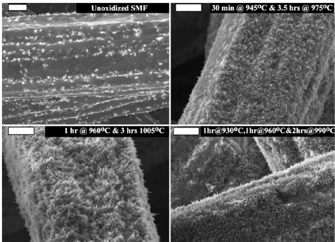
Figure 46: SEM micrograph of sintered micro fibers oxidized at various temperatures.<sup>320</sup> Copyright 2011 Elsevier.
