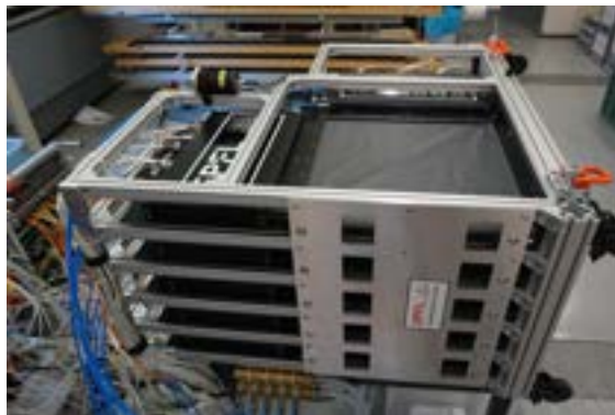
Figure 8. The SciFi tracker detector setup in the lab for cosmic ray test. The active area of a tracker module is 40 cm \times 40 cm and consists of 5 \times 5 fibre planes.
