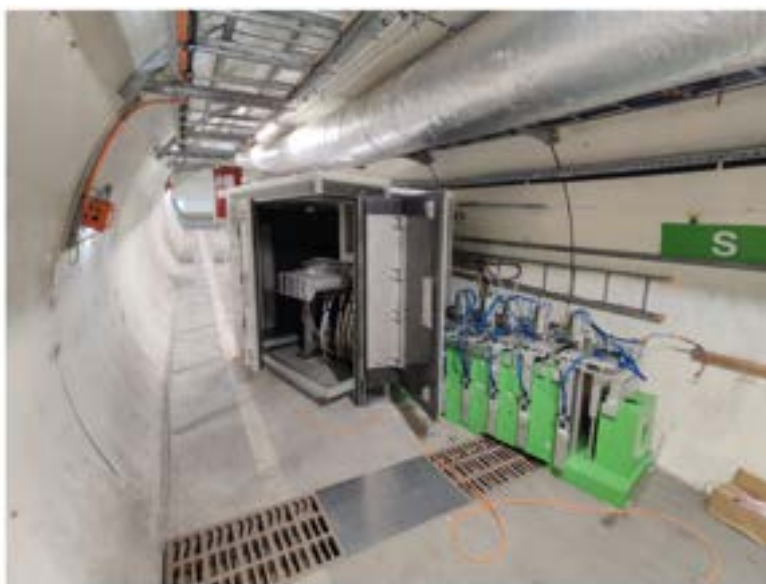
Figure 53. Global view of the detector in TI18 after the installation of the neutron shield.
