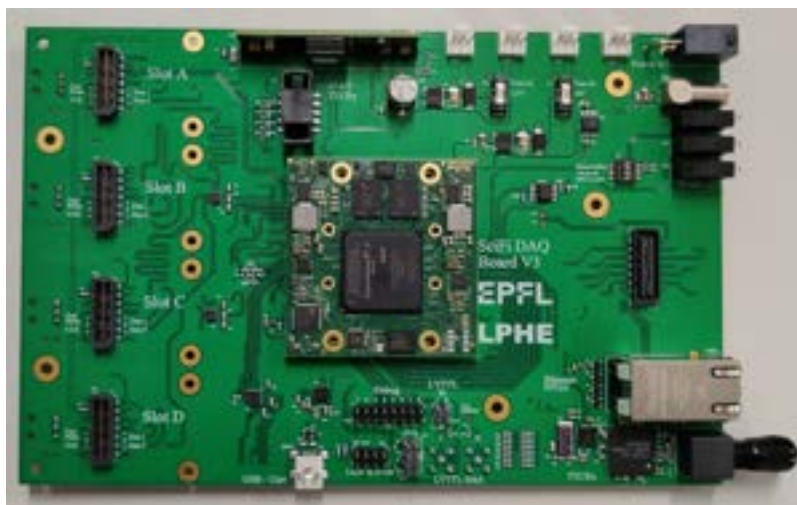
Figure 25. Photo of the DAQ board. The four FE board connectors are visible on the left, the TTCrx and optical receiver on the bottom-right, and the Enclustra Mercury SA 1 module in the centre.
