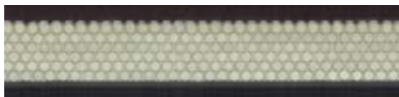
Figure 9. The fibre mat is composed of six layers of fibres glued with a titan oxide loaded epoxy glue to suppress cross talk between fibres.
