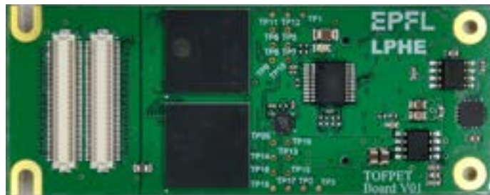
Figure 24. The FE board. The two TOFPET2 ASICS (centre) and the SiPM connectors (left) are visible.
