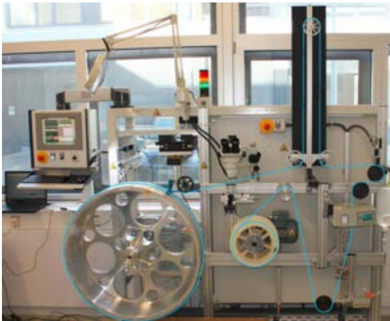
Figure 10. The winding wheel with a circumference of 2.5 m allows to wind five 40 cm mats. The winding process has been refined and adjusted in order to obtain precise and regular fibre mats. The path of the fibre in the machine is highlighted in cyan.
