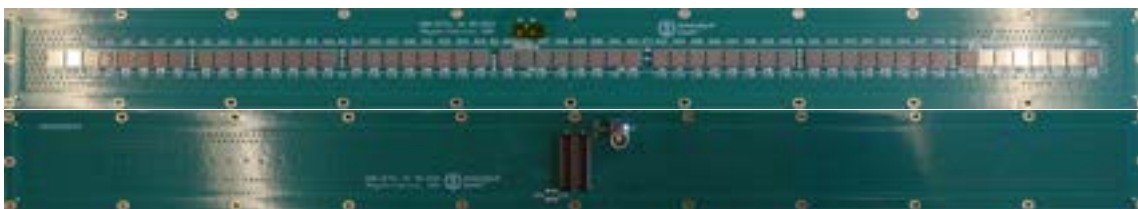
Figure 6. The two sides of the PCB for the veto system.
