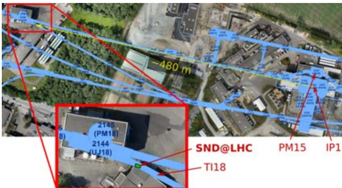
Figure 50. The location of the SND@LHC detector. SND@LHC is located in the TI18 tunnel, accessible from the LHC one via UJ18, 480 m from the ATLAS interaction point. Access can be performed via the PM15 and PM18 shafts.
