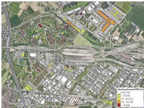
Fig. 4 | Pilastrò / Roveri district, Bologna: 3D model made with iCD; attribution to the buildings of the prevailing uses and building type, which contribute to estimating the energy consumption baseline (source: projectgreta.eu; r2msolution.com).
