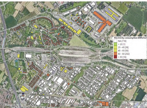
Fig. 4 | Pilastrò / Roveri district, Bologna: 3D model made with iCD; attribution to the buildings of the prevailing uses and building type, which contribute to estimating the energy consumption baseline (source: projectgreta.eu; r2msolution.com).
