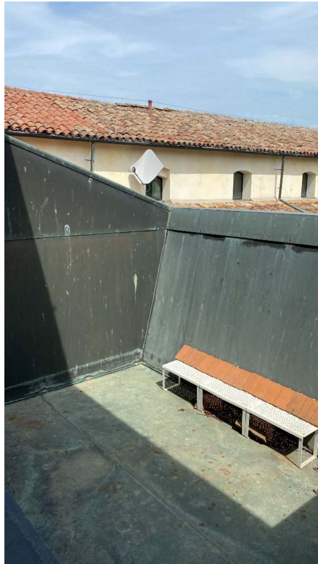
Fig. S5. Long-term outdoor ageing: general view of specimens exposed on a terrace at the Museo Internazionale delle Ceramiche in Faenza.
