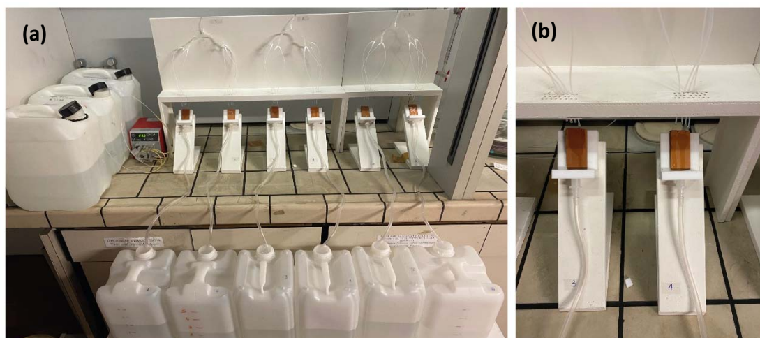
Fig. S3. Runoff test setup (a); detail of two runoff stations during the test (b).
