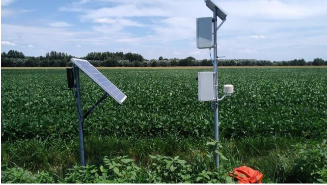
Fig. 1. Sensors installed at Ceregnano (Italy). The gSMS by Medusa on the left and CRNS by Finapp on the right.
