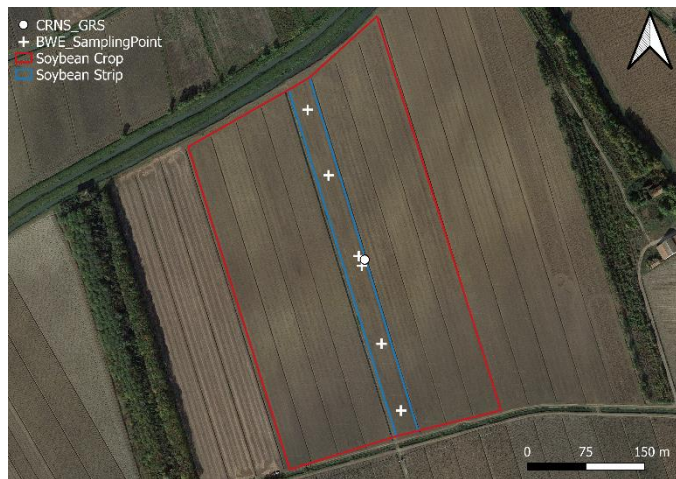
Fig. 4. Vegetation sampling pattern for biomass water equivalent determination and area of interest for NDVI estimation based on Sentinel 2.
