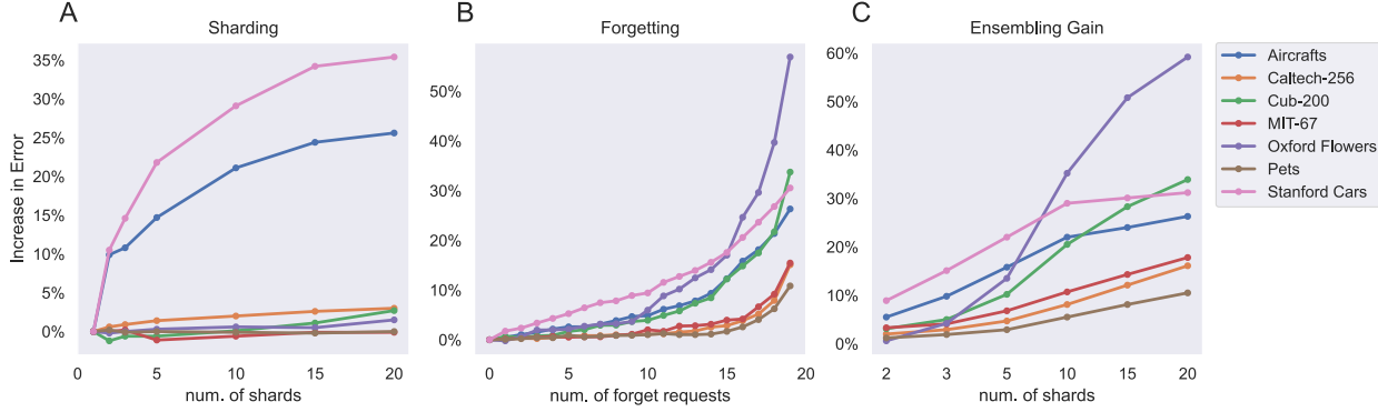
Figure 3. (A) Error increase of APT compared to paragon. We split a training set into a varying number of equal sized shards chosen uniformly at random. We then use APT to combine prompts learned individually on each shard, and measure the increase in error compared to the paragon of training on all data together. For most datasets, the performance of the APT is within a few percent of the paragon, even when the dataset is split in up to 20 parts. Aircrafts and Stanford Cars are the main exceptions, possibly due to the large domain shift between the backbone pretraining and those tasks. (B) Satisfying forgetting requests. We simulate a sequence of data removal requests starting from a pool of 20 sources and removing one source at the time. We report the increase in error compared to using the full data. We see that APT degrades gracefully as desired, while also ensuring perfect data removal. (C) Gain of using ensembles instead of individual prompts. We split a train set in a varying number of shards, and show the difference between the accuracy of APT prompt composition and the average accuracy of the individual prompts. For large number of shards, individual prompts don't have enough information to classify accurately but APT can combine them to create a much stronger classifier (with up to 60% better accuracy).
