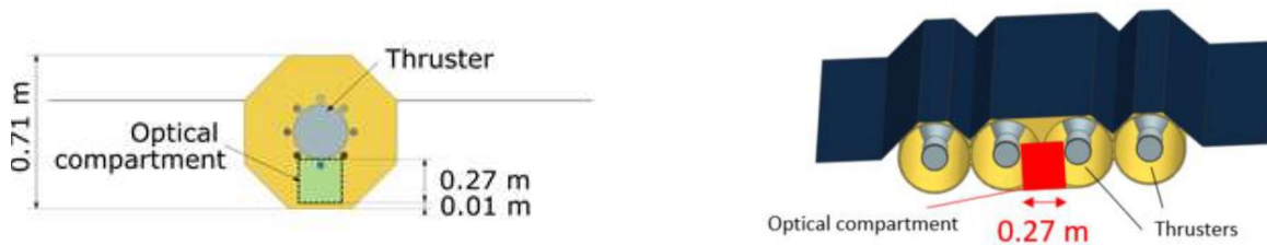
Figure 14. Back views of the slender body (left) and flat body (right) configurations, indicating the placement of the Earth observation payload's optical compartment.
