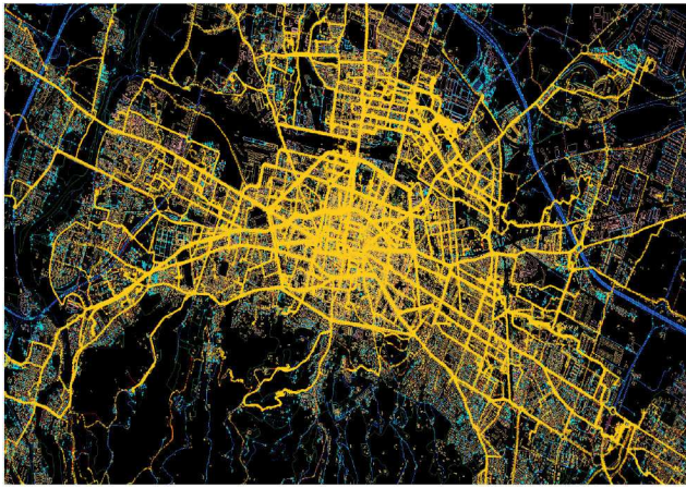
Fig. 2 Bologna SUMO transport network (in blue), overlapped with GPS traces from the ECC (yellow) recorded in 2015. The graphics are generated by the GUI from SUMOPy
