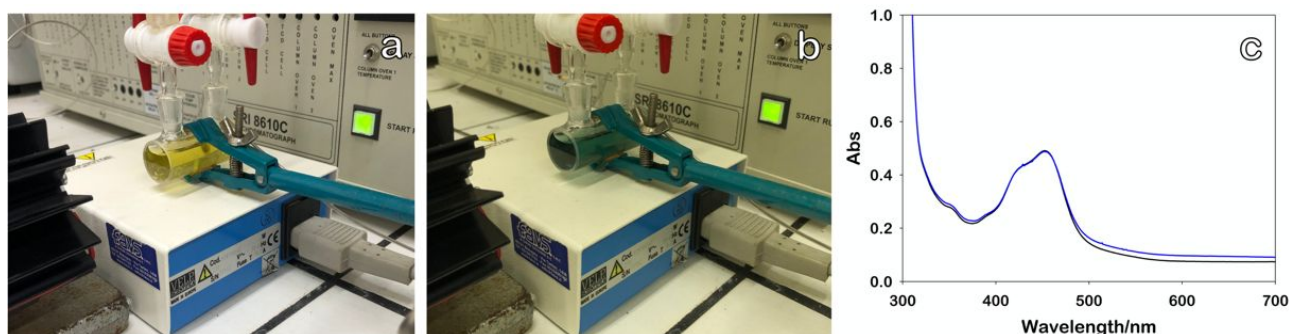
Figure S7. Reaction mixture before (panel a) and during (panel b) H 2 photosynthesis using RuO 2 in acetonitrile. Panel c shows absorption spectra before (black line) and after one hour irradiation (blue line).
