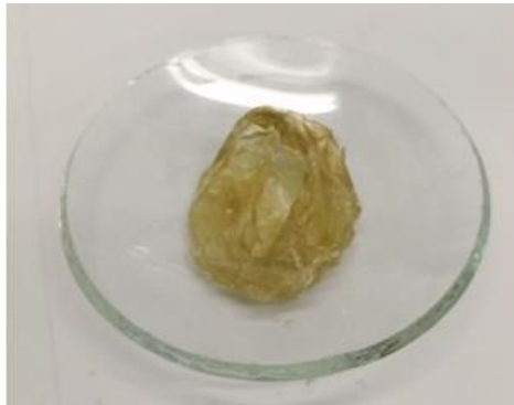
Fig. 7 – PHB extracted from D. communis biomass during the semi-continuous cultivation test.
