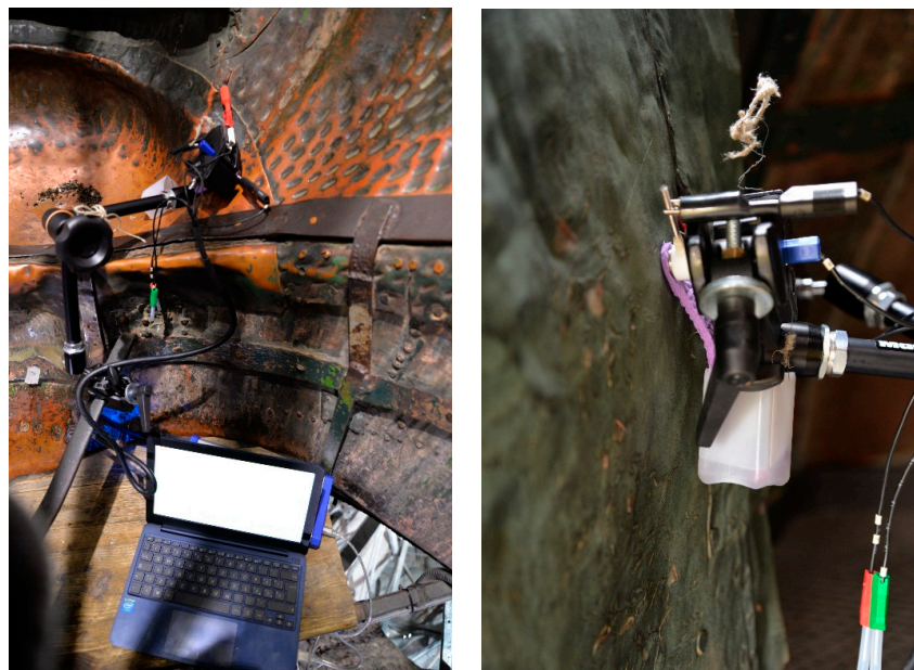
Figure 3. In situ electrochemical measurements with the contact probe.
