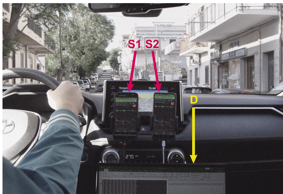
Figure 4. Smartphones used as sensing platform for detecting driving style: testing and validation (S1—Device to validate; S2—Reference device; D—Data acquisition).
