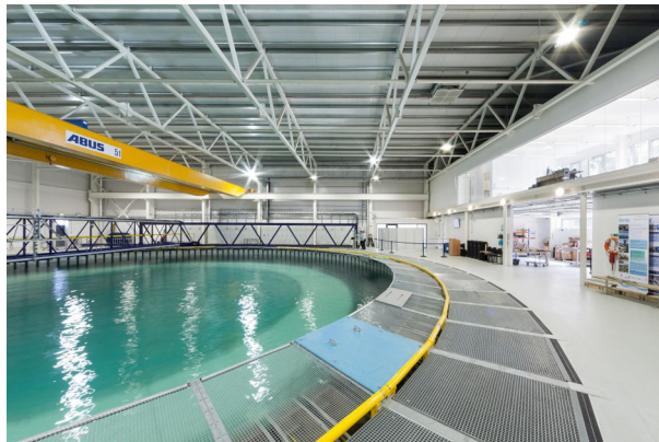
Fig. 1 The 25 m diameter circular facility FloWave at the University of Edinburgh
