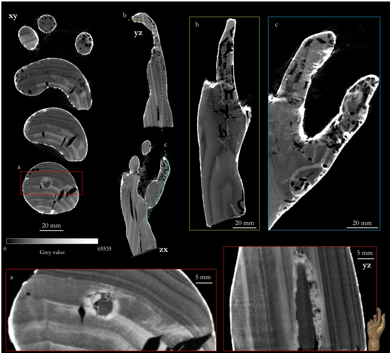
Fig. 9 X-ray tomography of the 13th-century statue's hand. Left: axial slices (xy) showing the alternating earlywood and latewood bands and, in the red box, the wrist area containing a wooden dowel likely used for the original joint with the forearm. Bottom: magnified axial and longitudinal views of the dowel (red boxes). Centre: sagittal (yz) and normal (zx) sections; lines b and c indicate the paths used for dynamic
