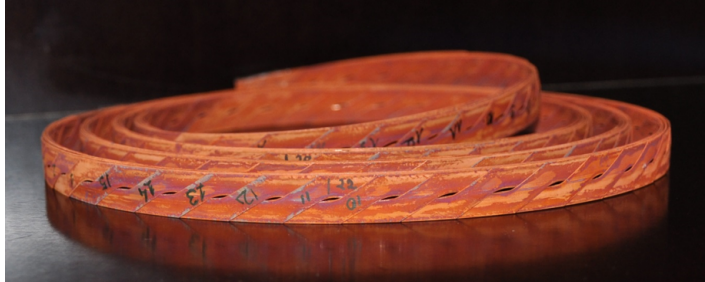
Figure 1: Roebel-based coil under investigation at the University of Southampton [20].
