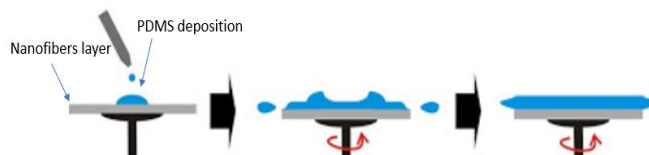
Fig. 4 Schematic principle of the spin coating process.
