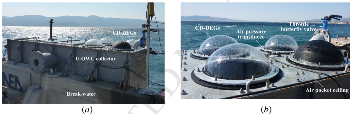
Figure 3. Metallic caisson incorporating the U-OWC (a) with, on the top, four CD-DEGs on the lateral chamber (b). The U-OWC/CD-DEG is connected to a vertical breakwater serving as a ballast for the system. One of the CD-DEGs has been painted black to facilitate post-processing of the high-speed camera frames.
