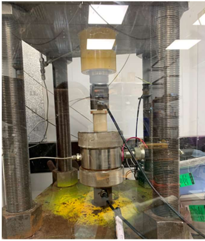
Figure S3.3. Schematic of the experiment. a : transducer in box holder with spring attached; b : jacketed rock sample; c : hydraulic uniaxial; d : sample chamber with confining stress; e : pressure control; f : Piston
