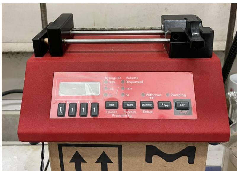
Figure S1: NE-1010 Higher Pressure Syringe Pump used to perform slow-addition of acetylenes
