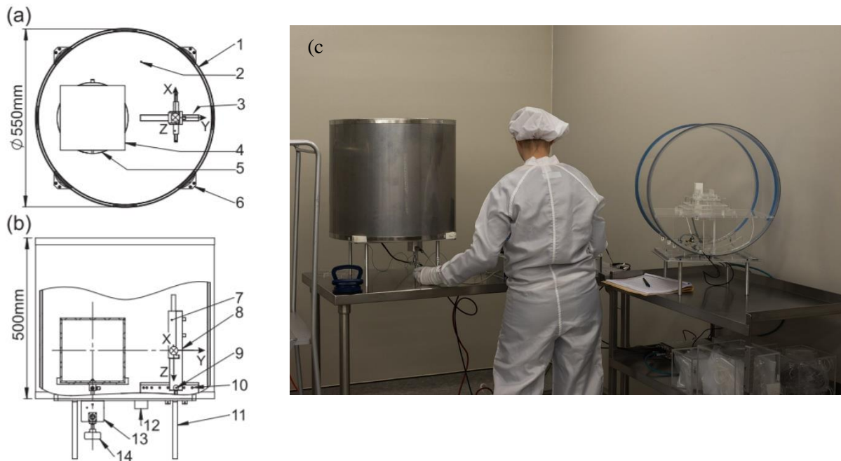
Figure S-1a. left. Schematic illustrations of the magnetometer in the top view opening the top cover (a) and the side view showing the interior by a broken-out section of the shield (S-1b). A two-layered mu-metal shield (1) enclosing a three-axis fluxgate sensor (7) mounted on a sensor holder (8) that can slide on a rail (3), and a sample (4) on a rotating table (5). The sensor-to-sample distance is adjusted by changing the position of the pin (9) fixed on bores (10). The user can rotate the table by a handle (14) and the rotation angle is measured by an optical encoder unit (13). The power supply and the outputs of the sensor are connected to the outer signal conditioning unit via feedthrough (2) and a connector (12). The mu-metal shield and the entire system is mounted on an aluminum plate (6) supported by aluminum feet (11). The coordinate system is shown in the figures. The horizontal and vertical lines in (S-1b) show rotation axis and the horizontal centerline of the sensor, respectively (Uehara et al., 2017) (S-1c) Three-axis fluxgate magnetic field sensor (Mag-03MS100, Bartington Instruments, Ltd.*) and a rotating sample stage with two-layer mu-metal magnetic shield (550 mm in diameter and 500 mm in height) (photo credit: Professor Ben Weiss). *The naming of this reference instrument is intended for planning and discussion purposes only. Instrument-level performance requirements, sufficient to conduct a competitive procurement, have yet to be written.
