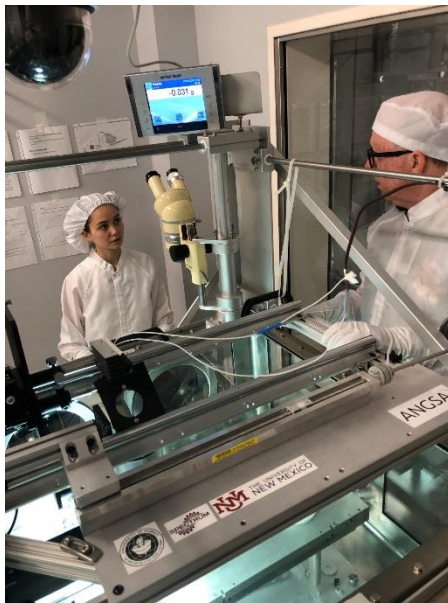
Figure S-5a (left). Multispectral and hyperspectral measurements in a glovebox of Apollo samples for ANGSA at the Johnson Space Center. Photo credit: Juliane Gross. S-5b (right). multispectral and hyperspectral comparison from https://www.edmundoptics.fr/knowledge-center/application-notes/imaging/hyperspectral-and-multispectral-imaging/
