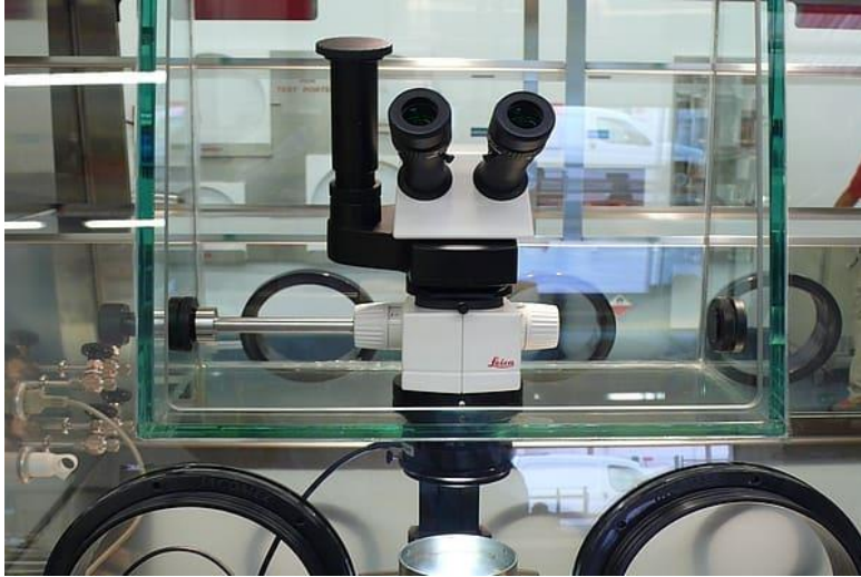
Figure S-4. Example of a Leica* binocular stereo light microscope attached to a glovebox.
