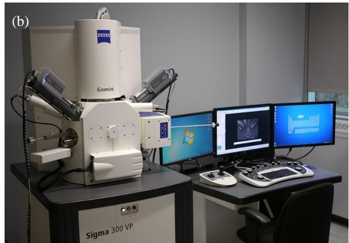
Figure S-7a (left). A Backscattered Electron Scanning Electron Microscope image of a polished thin section of a martian basalt photo credit: Carl Agee. S-7b (right). An example of such an instrument is a ZEISS Sigma 300 VP*, shown here from the University of Alberta. Console and operator's table is about 2 m wide and 1 m. A couple of feet from the instrument to the wall is needed for access, <230 kg. *The naming of this reference instrument is intended for planning and discussion purposes only. Instrument-level performance requirements, sufficient to conduct a competitive procurement, have yet to be written.
