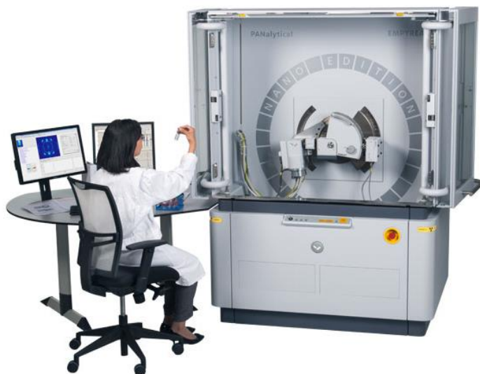
Figure S-22. An example of a Malvern Panalytical Empyrean powder X-ray diffractometer, Weight: 1400 kg, Exterior dimensions: 195 x 116 x 140 cm (full system). *The naming of this reference instrument is intended for planning and discussion purposes only. Instrument-level performance requirements, sufficient to conduct a competitive procurement, have yet to be written.
