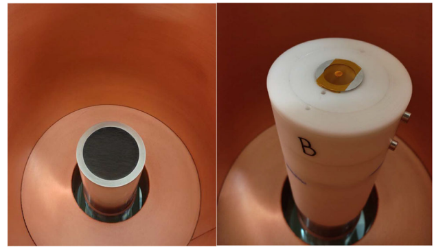
Fig. 10 Left panel: A view from the top of the HPGe detector inside the lead shield. Right panel: same as before, but with the polyethylene sample holder on top of the detector
