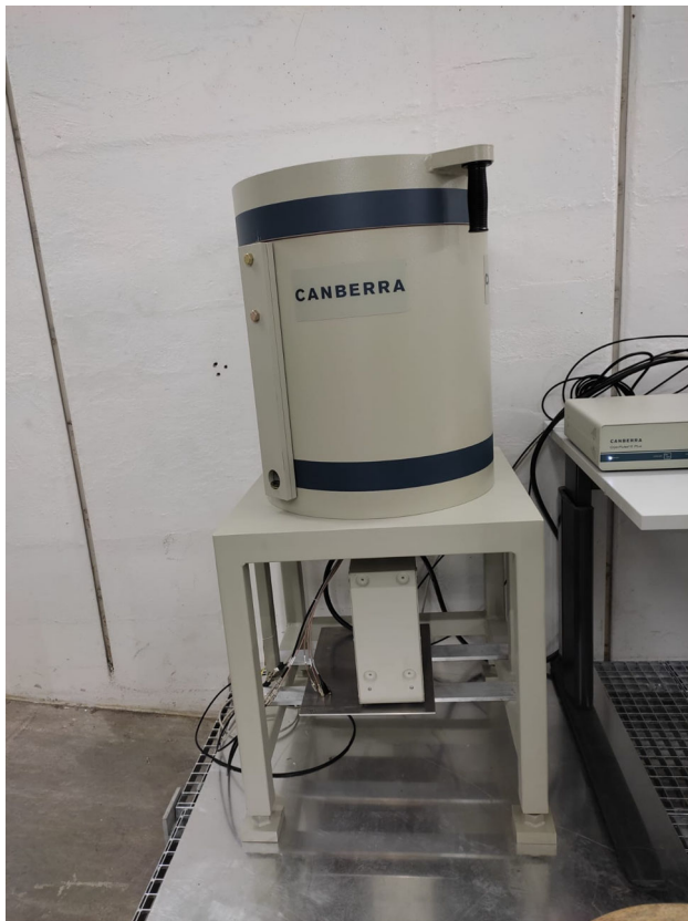
Fig. 9 The HPGe-based \gamma -ray spectrometer, placed in the GEAR Station. The detector is inside the lead shielding shown in the photo, while the refrigeration and front-end electronics are located underneath the shielding
