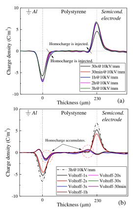
Figure 2. Space charge profiles of PS at 10 kV/mm: (a) polarization, (b) depolarization.
