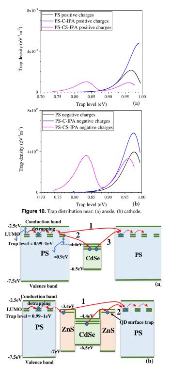
**Figure 11.** Simplified energy level diagram of PS (a) with core QDs, (b) with core-shell QDs.
