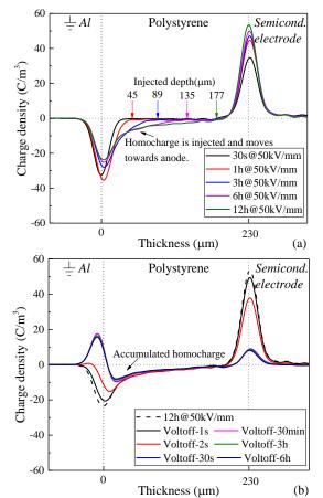
Figure 5. Space charge profiles of PS at 50 kV/mm: (a) polarization, (b) depolarization.
