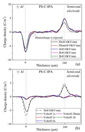
**Figure 4.** Space charge profiles of PS-C-IPA at 10 kV/mm: (a) polarization, (b) depolarization.
