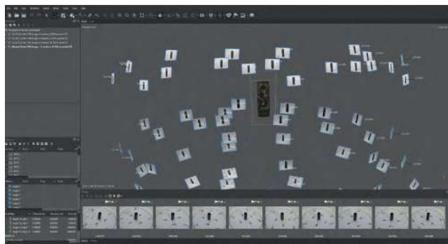
Fig. 1. Photogrammetric model of cylinder seal YU.25.O.5 from the necropolis of Yunus produced using Agisoft Metashape©.
