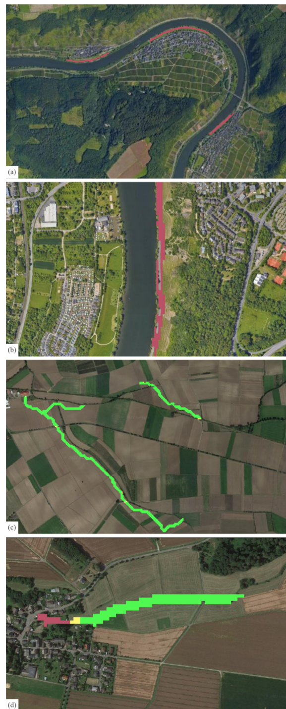
Figure 5. Results from satellite imagery validation: (a) red marked areas presenting potential riparian forest buffers suggested by the OSM-based suitability map, but not by the other two outputs (coordinates: 4120537 3005590: 4124094 3007762); (b) red areas present non-appropriate suggested areas by the CLC-based suitability map, but not by the other two outputs (coordinates: 4146529 3027011: 4147856 3027821); (c) inaccuracy of input and output layers (coordinates: 4191466 2963021: 4194514 2964882); (d) the general agreement of all output layers is marked in green, while yellow presents the agreement of two layers, and red is only one layer (coordinates: 4162673 3014443: 4163541 3014973).
