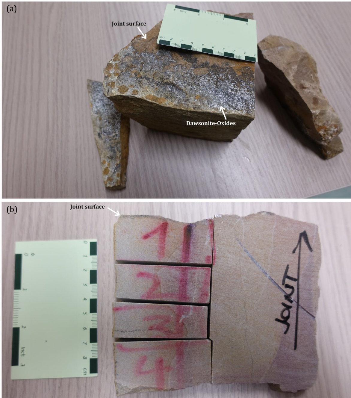
Figure S1. Poggio del Gatto sandstone from Mt. Amiata, Italy. (a) Top view with Dawsonite and oxide phases. (b) Side view showing thin-section sampling positions "Layer 1" to "Layer 4" at increasing distance from the joint surface.
