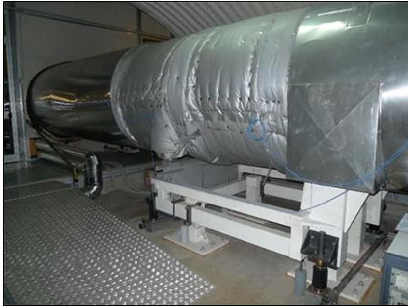
327 Figure 10. End Building-Tunnel link module. Special tube support with micrometric mechanical 328 realignment system.
