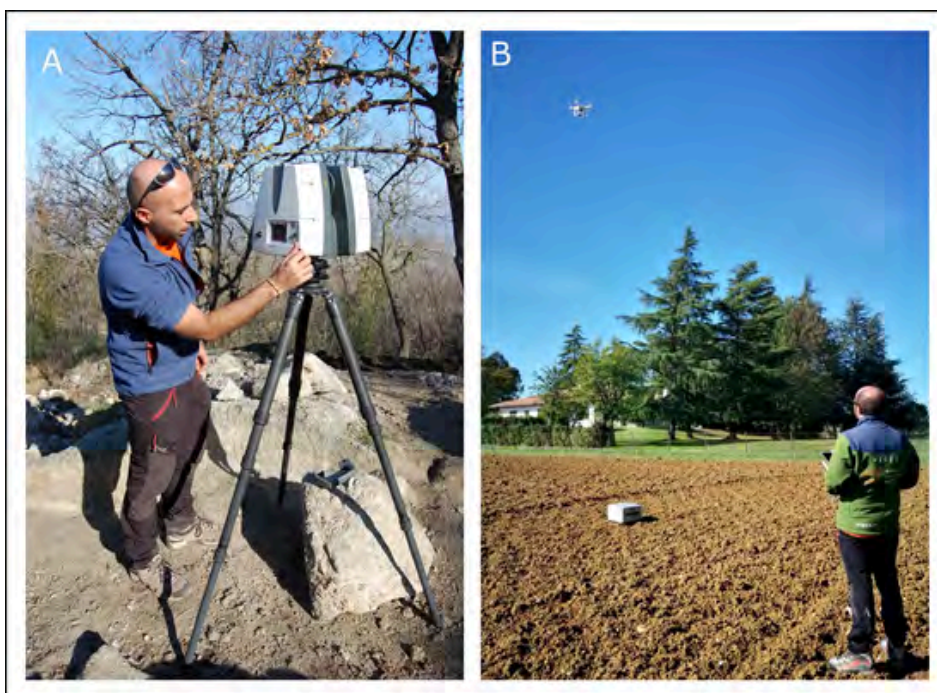
Fig. 3. A. The Leica P40 Scan Station during the survey in the Roman quarry; B. Operation of the DJI Phantom 4 Drone (circle) equipped with a digital camera for the realization of a digital model based on 147 digital images.
