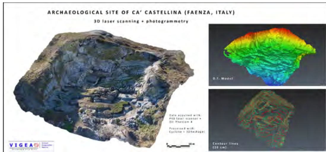
Fig. 4. Aerial photo (left), obtained using 147 drone-based photographs and digital terrain model (right up) and contour lines of the Roman quarry based on 17 laser scan station measurements.
