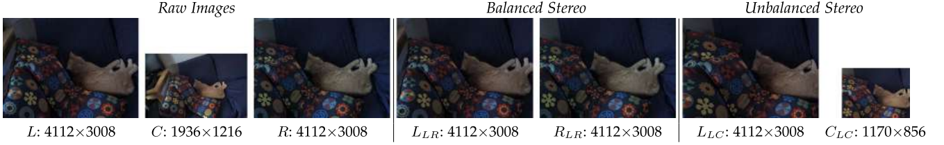
Fig. 4. Balanced/unbalanced rectification examples. From left to right: L , R , and C raw images from our rig; L_{LR} , R_{LR} rectified balanced stereo pair from the L - R setup; L_{LC} , C_{LC} unbalanced rectified stereo pair from the L - C setup.
