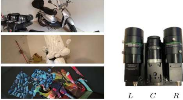
Fig. 3. Cameras setup and acquisition. On the left: i) passive stereo pairs collection, ii) painting of reflective/translucent materials, iii) textured stereo pairs acquisition. On the right, top-view of our camera rig, with L and R being two 12 Mpx sensors, and C a wide-angle 2.3 Mpx sensor.
