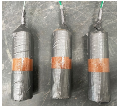
Fig. 5: sensorized ceramic elements wrapped with plastic film and insulating adhesive tape during the calibration phase.
