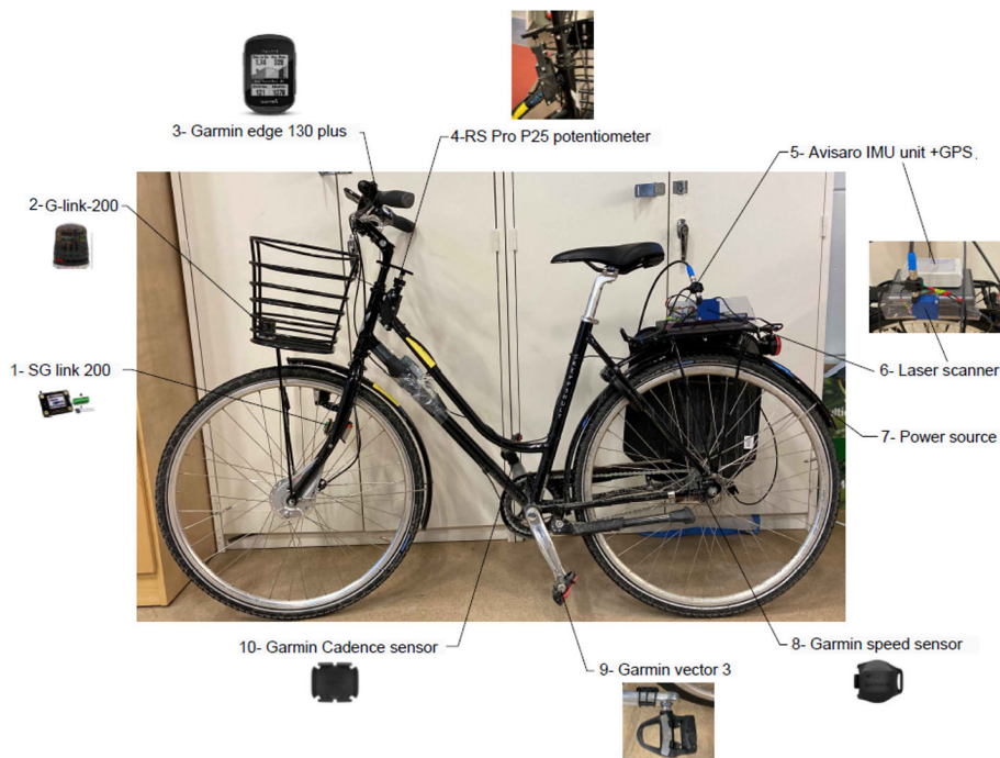
FIGURE 2. Schematic of the instrumented bicycle, more details about the different sensors following the correspondent numbers below.
