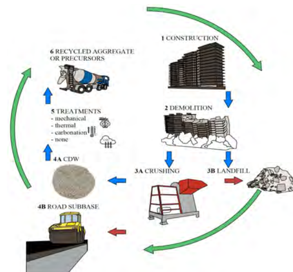
Figure 4. Construction and demolition waste cycle in the building industry. The green arrows represent the recycling process, the blue arrow represents an individual process phase, whereas the red arrow indicates a stage at which CDW exits the recycling process described in this review.
