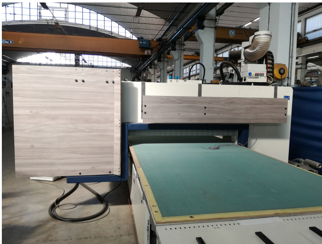
FIGURE 2. Configuration of the 9 US sensors mounted on the machine. The sensors are the grey metal round elements on the panels; the circular black pieces are washers for fastening the panels. Compare with Fig. 3.
