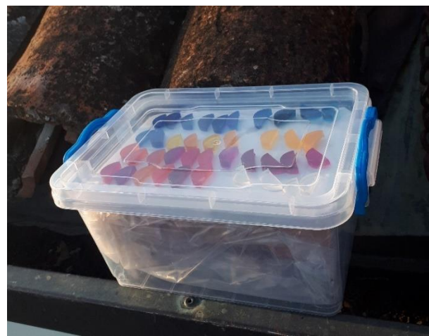
Fig. 4 Samples during the outdoor ageing period
