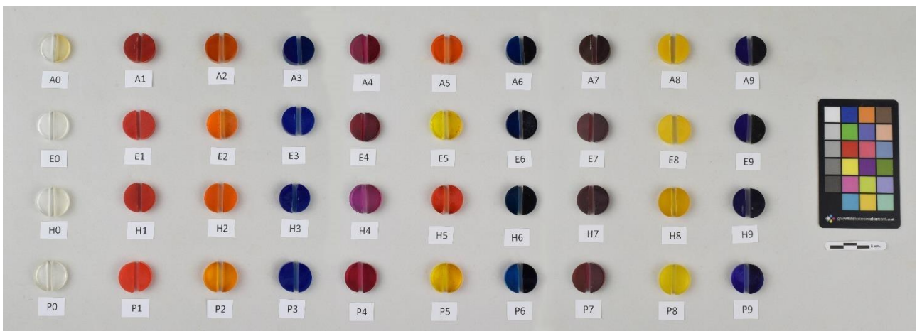
Fig. 6 Samples aged outdoor, on the left the non-exposed half, on the right the aged one. Colour differences can be seen.
