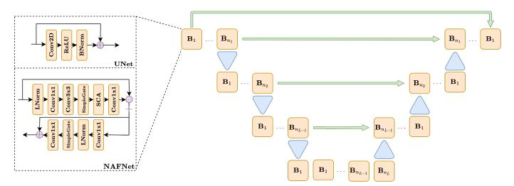
Figure 2. A diagram representing the UNet and NAFNet architectures.
