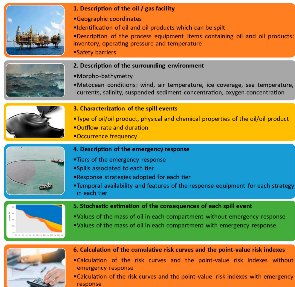
Figure 1. Steps of the methodology for the calculation of the risk indexes for environmental contamination caused by oil spills.
