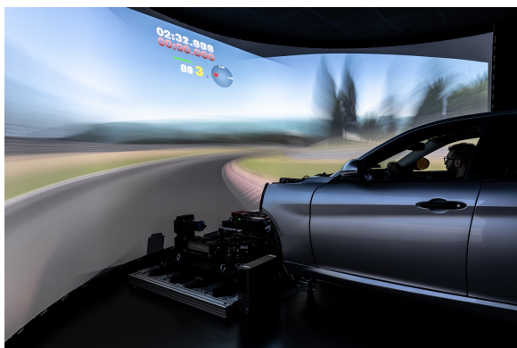
Fig. 2: Static driving simulator of Maserati company [13].
