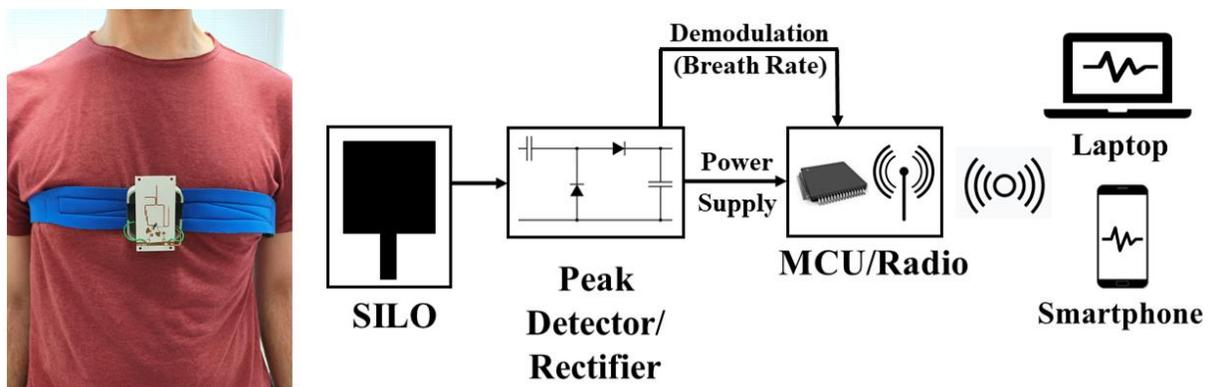
Envisioned scenario for the wearable sensor aiming at normal and deep breath rate detection, working at 5.8 GHz, and able to harvest energy for feeding a commercial microcontroller unit.
