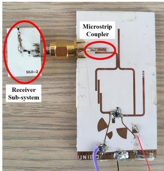
Fig. 9. Photograph of the breath sensor prototype, showing the connection of the oscillator output port to the receiving sub-system by means of a microstrip coupled line.
