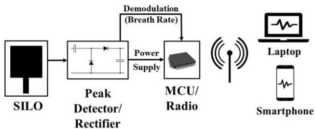
Fig. 1. An envisioned scenario of the wearable sensor for breath rate detection working at 5.8 GHz, able to detect human breath rate and to harvest energy for feeding a commercial SoC.
