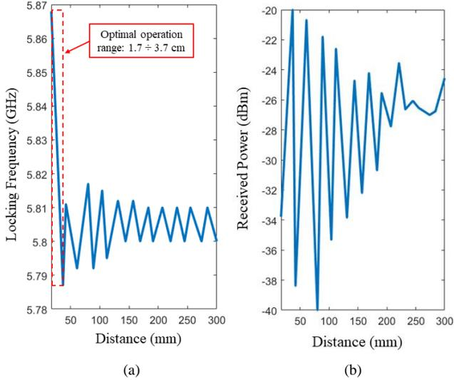
Fig. 6. (a) Locking frequency and (b) power received from the horn during displacement measurements of the oscillator antenna from a metallic reflector, for distances  $\Delta s$  ranging from 16 to 300 mm.
