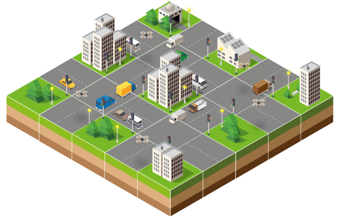
Fig. 8. A multi-tier IoV network comprised of moving cars, drones and traffic intersections equipped with sensing and communication capabilities. In this envisaged scenario communication takes place amongst entities in a multi-hop fashion. Cars could exploit the IoVs sensing capabilities, gathering and merging information from different complementary sources in order to extend the drivers' perception beyond direct line of sight.
