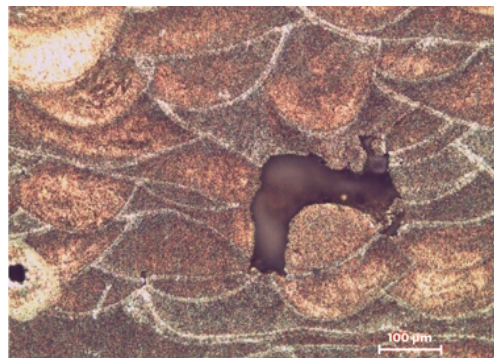
Figure 16. Porosity in a longitudinal section.
