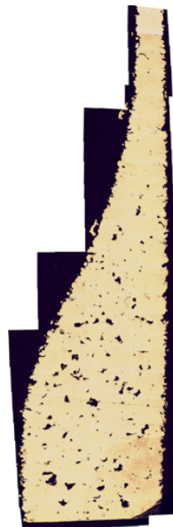
Figure 14. Porosity in a 1.2 specimen longitudinal section due to low energy density.
