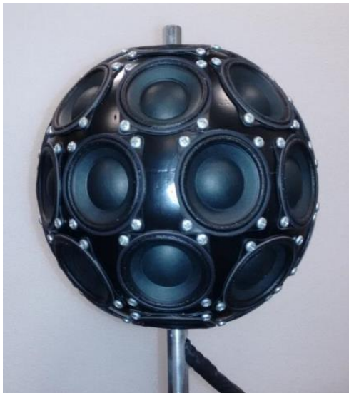
Figure 5: Prototype spherical array loudspeaker [3]
