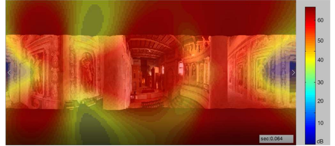
Fig. 6-10: Frames of the sound energy animation of measurement point 1 (pit)
