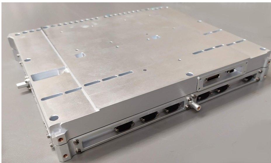
Figure 4. The LV-PS unit fully assembled. The overall dimensions of the unit are 29.8 cm × 24.3 cm × 4.0 cm.
