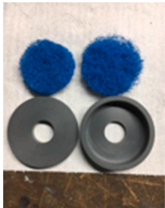
Fig. 13. The two demisters used in the experimental test.
