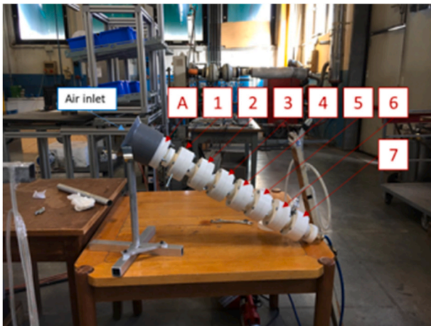
Fig. 4. The first tunnel to be built for the experimental campaign.
