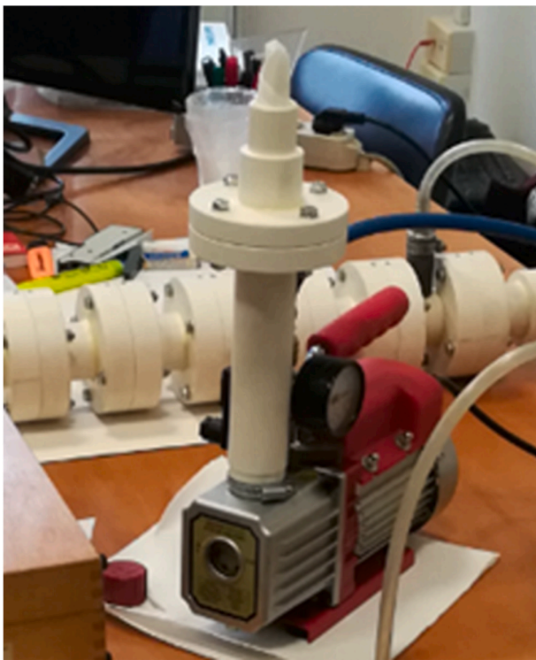
Fig. 5. The downstream chimney installed on the NPAV30 vacuum pump.
