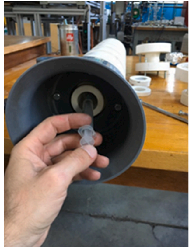
Fig. 3. A detail of the aqueous solution's entry point and of the protective collar.
