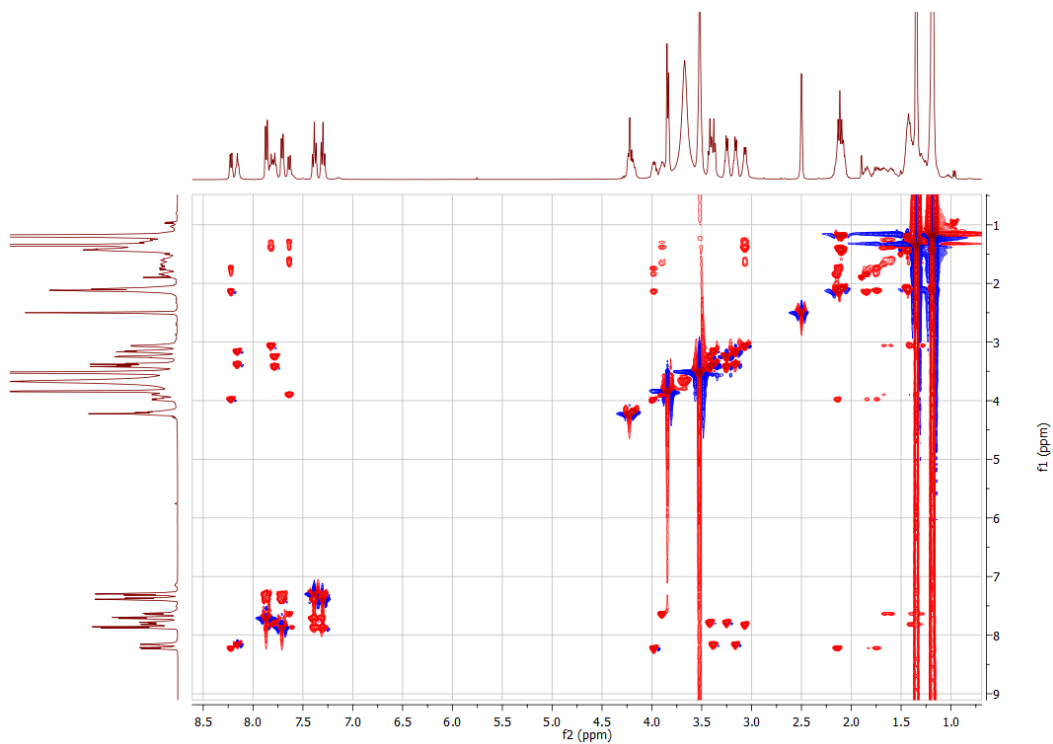
Figure S12. TOCSY spectrum of Tirzepatide SCBB after addition of 4 equiv. of \text{MgCl}_2 (400 MHz, \text{DMSO-}d_6 ).
