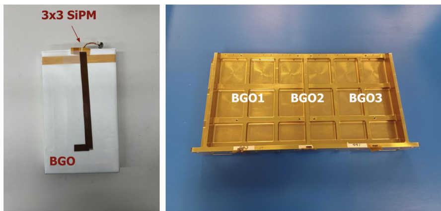
Fig. 2 Wrapped BGO crystal with coupled SiPM array on the left (picture taken at NRL) and the EM X-wall with the three BGO crystals on the right (picture taken at SSL)
