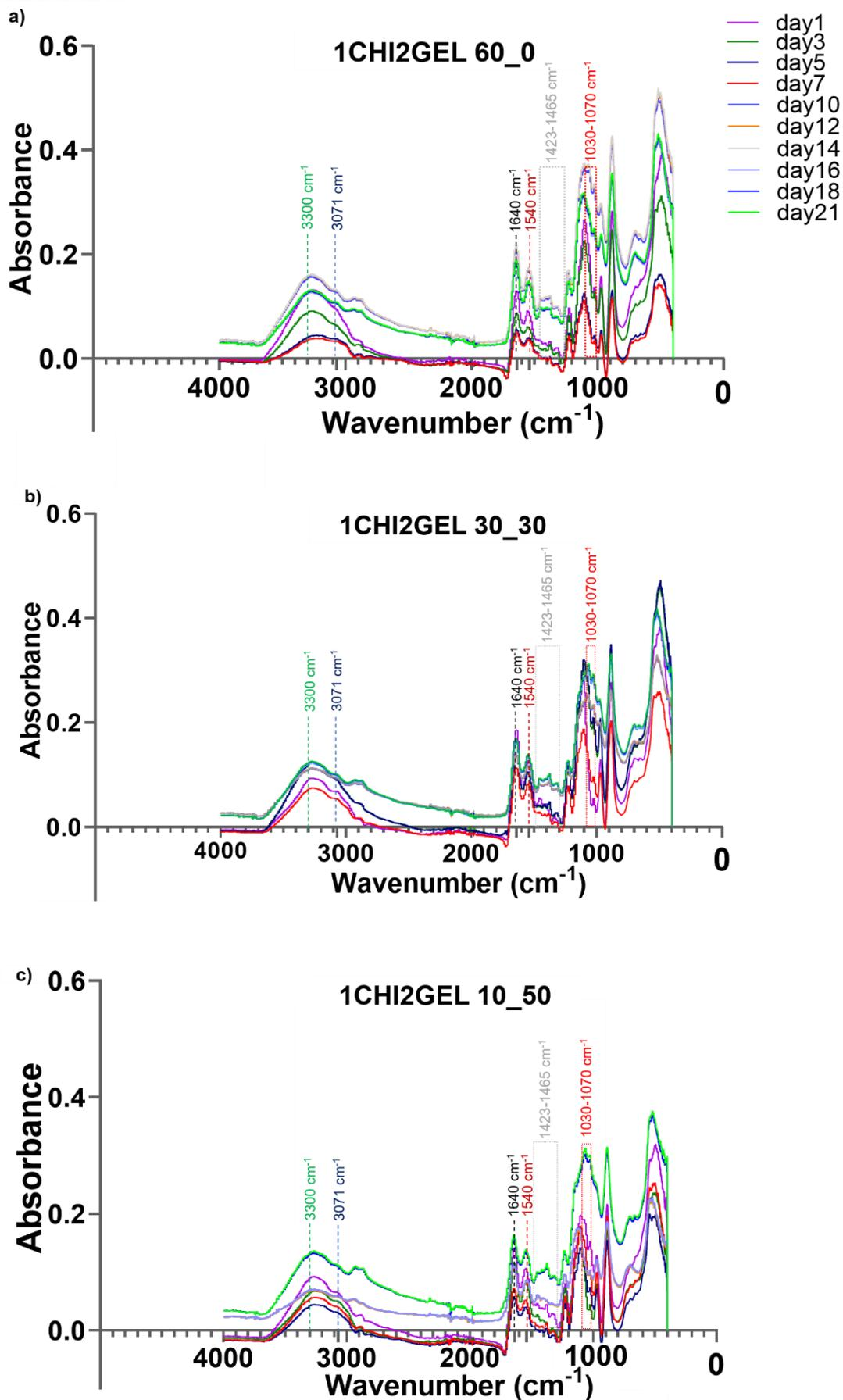
**Figure S2.** FTIR spectra for each crosslinking conditions (60\_0, 30\_30, 10\_50) of 1CHI2GEL 3D structures at different time points (1, 3, 5, 7, 10, 12, 14, 16, 18, 21 days). (a) 1CHI2GEL 60\_0 3D printed structure, (b) 1CHI2GEL 30\_30 3D printed structure, (c) 1CHI2GEL 10\_50 3D printed structure.
