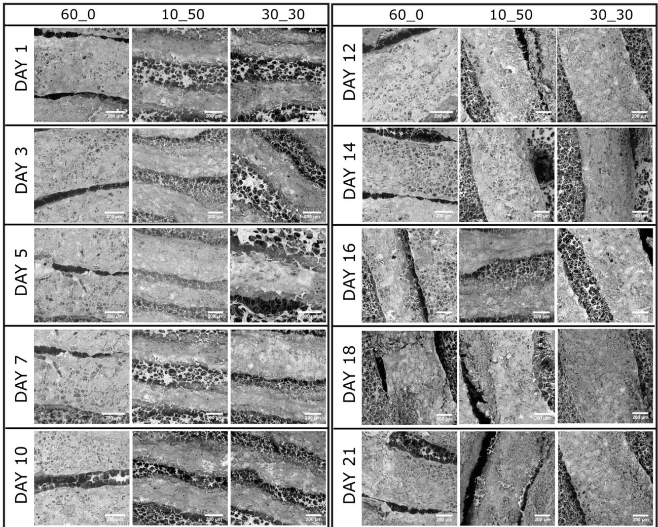
**Figure S4.** SEM images of fibers for each crosslinking conditions (60\_0, 30\_30, 10\_50) of 1CHI2GEL 3D structures at different time points (1, 3, 5, 7, 10, 12, 14, 16, 18, 21 days). (Scale bar: 200 $\mu$ m).
