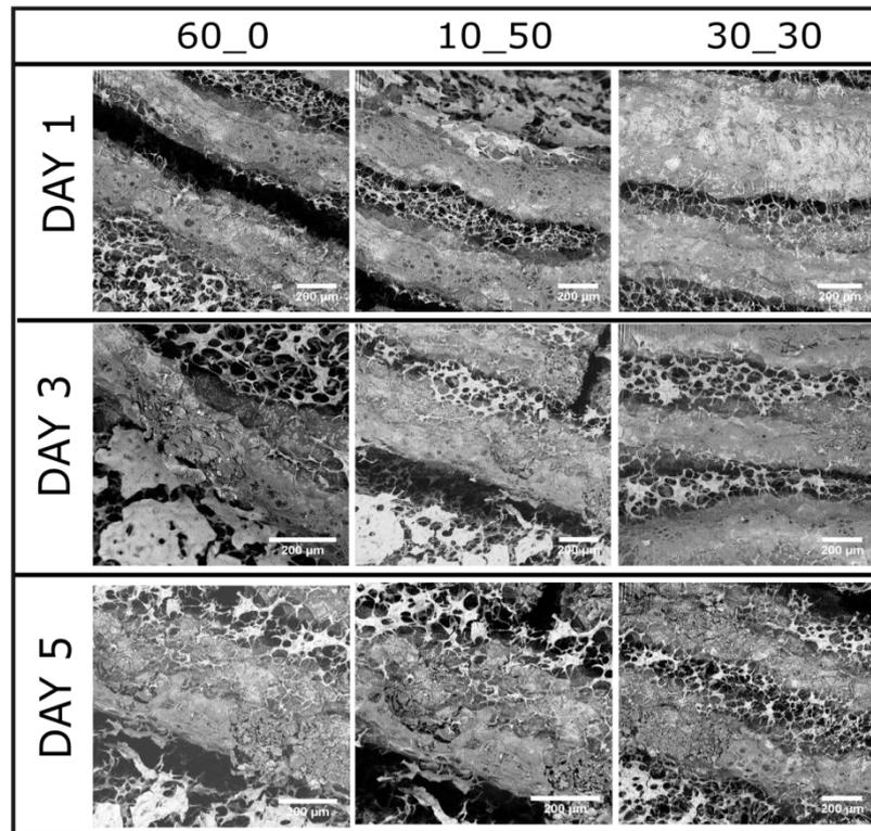
**Figure S5.** SEM images of fibers for each crosslinking conditions (60\_0, 30\_30, 10\_50) of 1CHI3GEL 3D structures at different time points (1, 3, 5 days). (Scale bar: 200 $\mu$ m).
