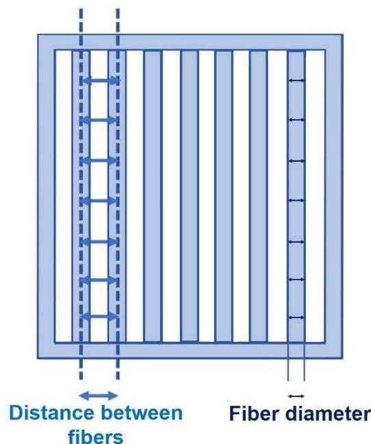
**Figure S1.** Measurement of fiber diameter and distance between fibers, calculated as the distance comprised between the axis of two adjacent fibers.
