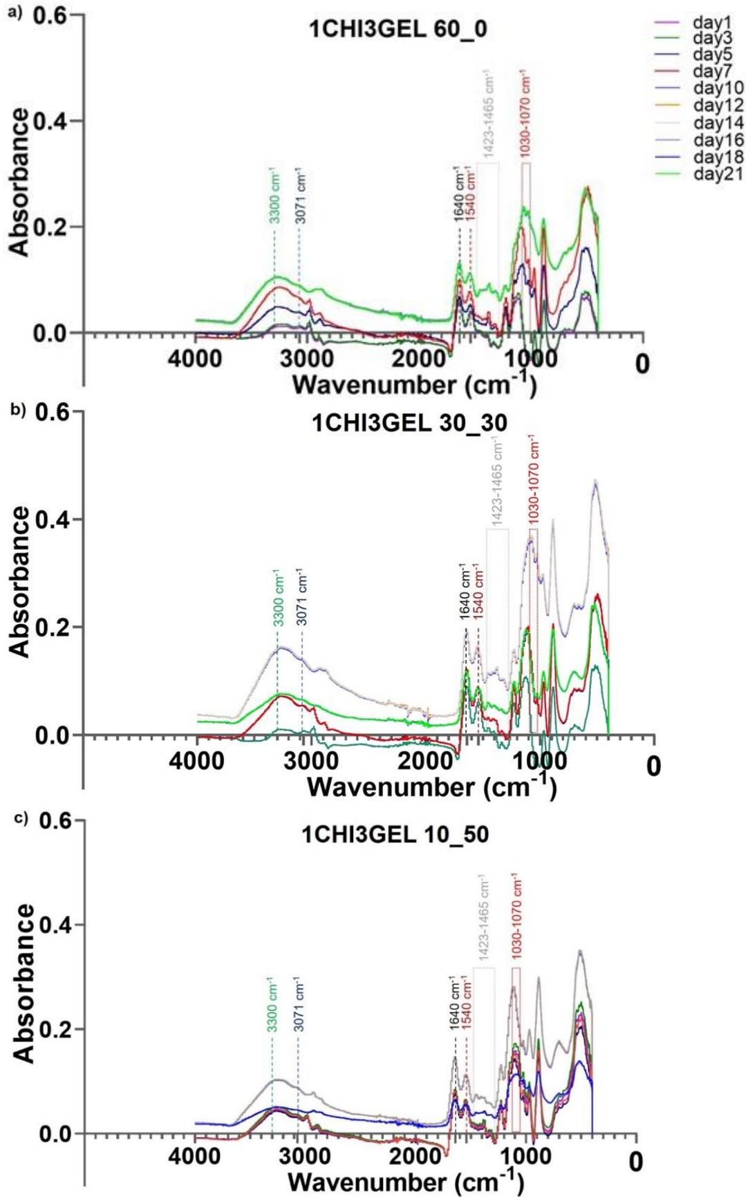
**Figure S3.** FTIR spectra for each crosslinking condition (60\_0, 30\_30, 10\_50) of 1CHI3GEL 3D printed structures at different time points (1, 3, 5, 7, 10, 12, 14, 16, 18, 21 days). (a) 1CHI3GEL 60\_0 3D printed structure, (b) 1CHI3GEL 30\_30 3D printed structure, (c) 1CHI3GEL 10\_50 3D printed structure.
